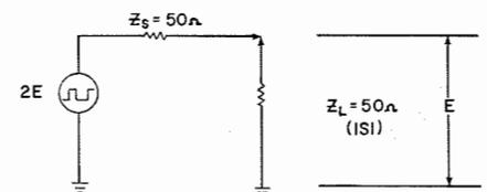
Figure 3. Simplified equivalent circuit representing the Amplitude Calibrator of a Type 544, Type 546, or Type 547 Oscilloscope and a Type 1S1 Sampling Unit.
