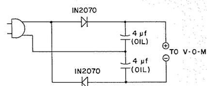
Figure B. Peak-to-peak reading adapter for 20,000 ohm/volt V-O-M. The use of silicon diodes and oil-filled (or Mylar, or paper) capacitors assures accurate voltage output.
