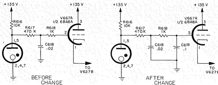
Figure 4. Before and After schematics showing installation of 0.1 discap in the +135 V supply of the Type 125.
