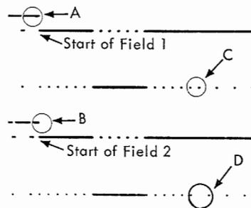
Figure 2. Waveform display showing that *Field One* is preceded by a full line of video (A) and *Field Two* by a  $\frac{1}{2}$  line of video (B). (C) and (D) indicate the equalizer pulses in the vertical blanking interval that determine correct instrument triggering.
