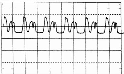
Figure 1. Typical oscillation waveform, caused by conditions described in text, displayed on a Type 547 Oscilloscope. Sweep rate  $0.1 \mu\text{s}/\text{cm}$ . Waveform will be different on Type 545 (A), (B) Oscilloscopes but fundamental frequency will still be about 10 MHz.
