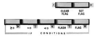
tects whether the flag is set, and another detects whether the display is flashing as caused, for example, by taking the square root of a negative number. Thus, the FLASH key can be used to detect whether the roots of a quadratic equation are real or complex.
