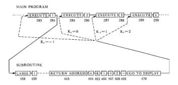
Here the stored return address is 285, but a value of  $K_1$  other than 0, either established before executing subroutine 1 or else established by logic within subroutine 1 causes the subroutine to branch back to the main program at locations other than 285.
