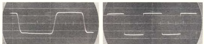
Fig. 1. 1 megacycle square wave. Fig. 2. 60 cycle square wave. Response of 2 Stage Vertical Amplifier.
