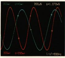
Another feature of the 5116 with the 5D10 is a direct readout of frequency or  $1/\Delta T$  (see display where  $1/\Delta T = 933$  Hz). This is one less step for you to get your measurement results.
