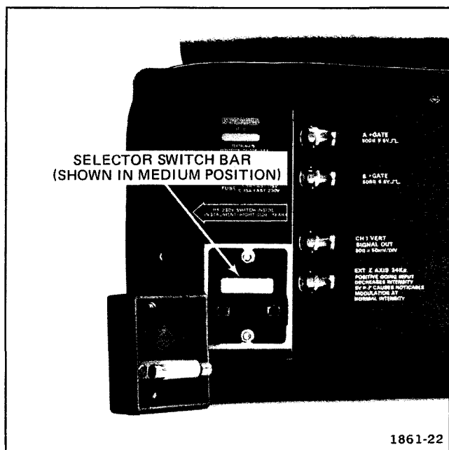
Fig. 2-1. Power supply regulating range selector.
