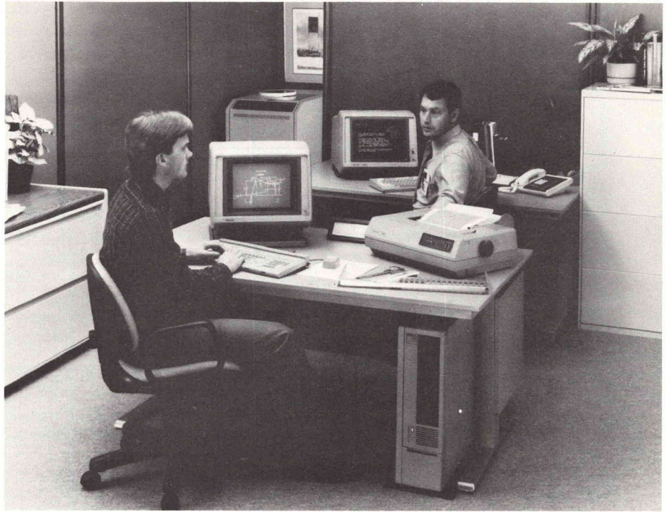
The 6130 Intelligent Graphics Workstation is designed for computer-aided engineering applications. The 6130 is shown here with a 6000 Family display (in the foreground), a 4107 computer display terminal (in the background) and a 4695 Color Graphics Copier.
