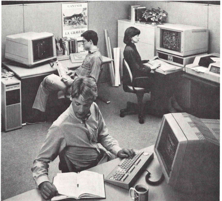
The 6200 Series Intelligent Graphics Workstations combine substantial computer power, mass storage and a Local Area Network (LAN) interface, making them suitable for ME design and analysis as well as large-scale ECB, custom VLSI or gate array design. Shown here is the Tektronix 6212 connected to the 6000 Family high performance display, 4115B and 4107 Computer Display Terminal .
