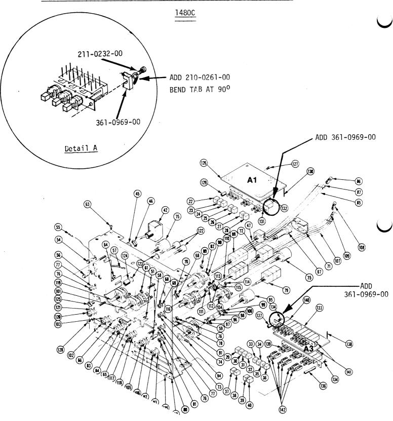
SPACER ADDED TO INSIDE OF SWITCH ASSEMBLY. SEE <u>DETAIL A</u> FOR EXACT LOCATION. CHANGE (6) MOUNTING SCREWS FROM 211-0268-00 TO 211-0232-00.
