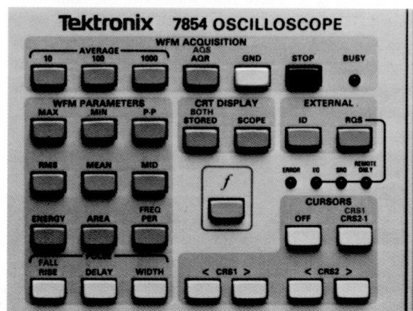
Fig. 3. Most waveform digitizers have some means of zero referencing acquisitions. This can be by either issuing a command to the instrument or pressing a ground acquisition button (GND) with the input channel switched to ground.
