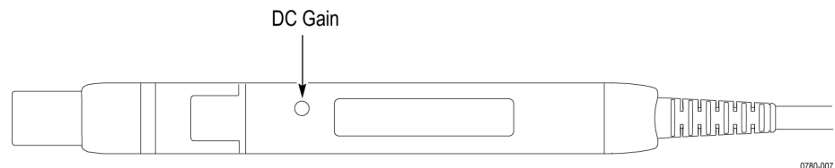
Figure 15: TCP305A and TCP312A DC gain adjustment location
