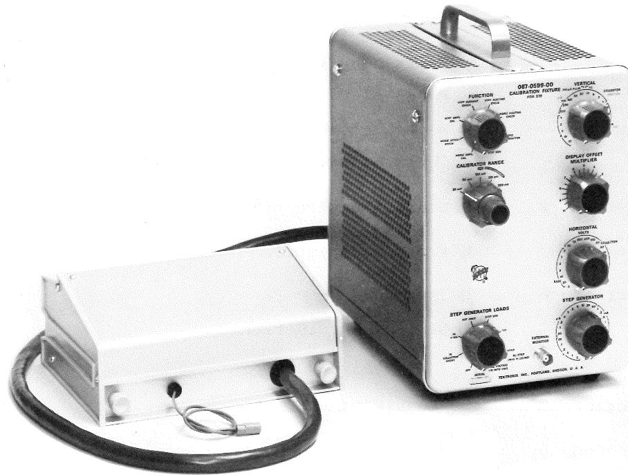
The 067-0599-00 Calibration Fixture was designed specifically for calibrating and testing the performance of the 576 Curve Tracer.
