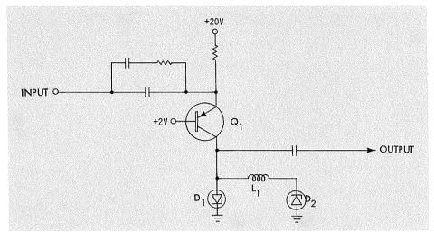
Figure 1 Typical Sampling Trigger Circuit.
