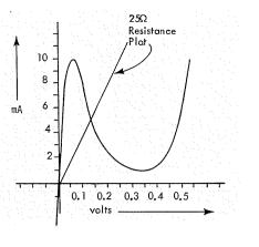
Figure 7 25-Ω resistance plot on a 10-mA tunnel-diode curve.
