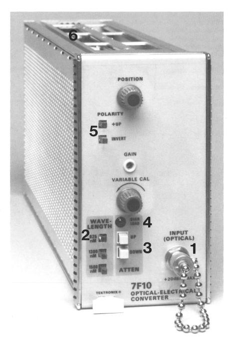
The 7F10 plug-in module is an optical to electrical converter for use with either single mode or multimode fibers. It offers 10 kHz to 750 MHz frequency response and covers the 700 to 1550 nanometer spectrum. It is designed mainly for use in vertical compartments of 7000 Series Oscilloscopes. It converts a 7000 Series mainframe into an optical oscilloscope.
