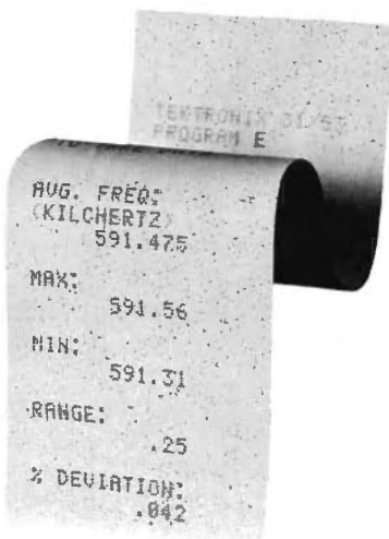
Fig. 1. Tape readout from an actual test of oscillator performance. Average frequency and minimum and maximum frequencies are readily measured and recorded.
