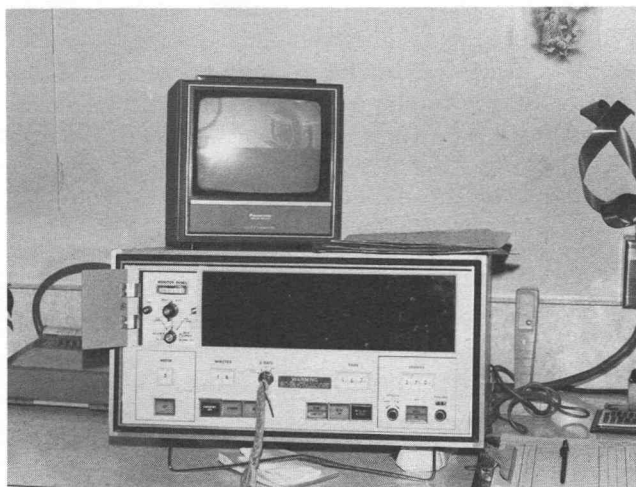
Fig. 5. The console controls radiation and the closed circuit television monitors the patient.
