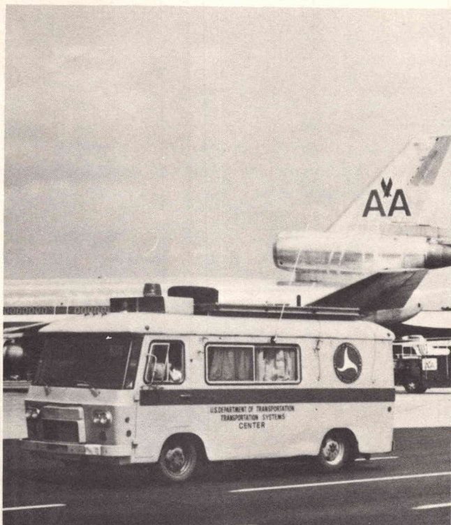
Fig. 1 Traversing the highways with their mobile data acquisition van, which includes a 4051 Graphic System, the U.S. Department of Transportation is evaluating the use of LORAN-C signals for on-land site location.
