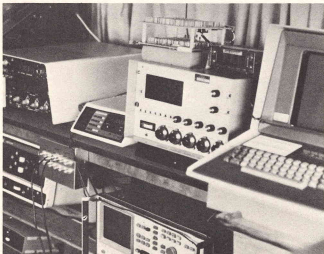
Fig. 3 The 4051 Graphic System controls data acquisition in the DOT van. LORAN-C receivers acquire the signals.
