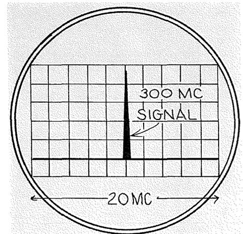
Figure 3. Dispersion, or bandwidth, set at 20 Mc. Each cm = 2 Mc.
