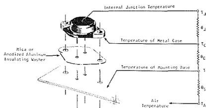
Figure 1. Electrical analog of heat path in a heat-sinked transistor.  $\theta_{jc}$  = Thermal resistance of junction to case bond. (Controlled by manufacturing process only.)  $\theta_{cs}$  = Thermal resistance of mounting. (Silicone grease can improve surface contact between transistor and mounting surface.)  $\theta_{sa}$  = Thermal resistance of "heat sink" or mounting base. (Usually a designed in factor after other elements have been optimized.)
