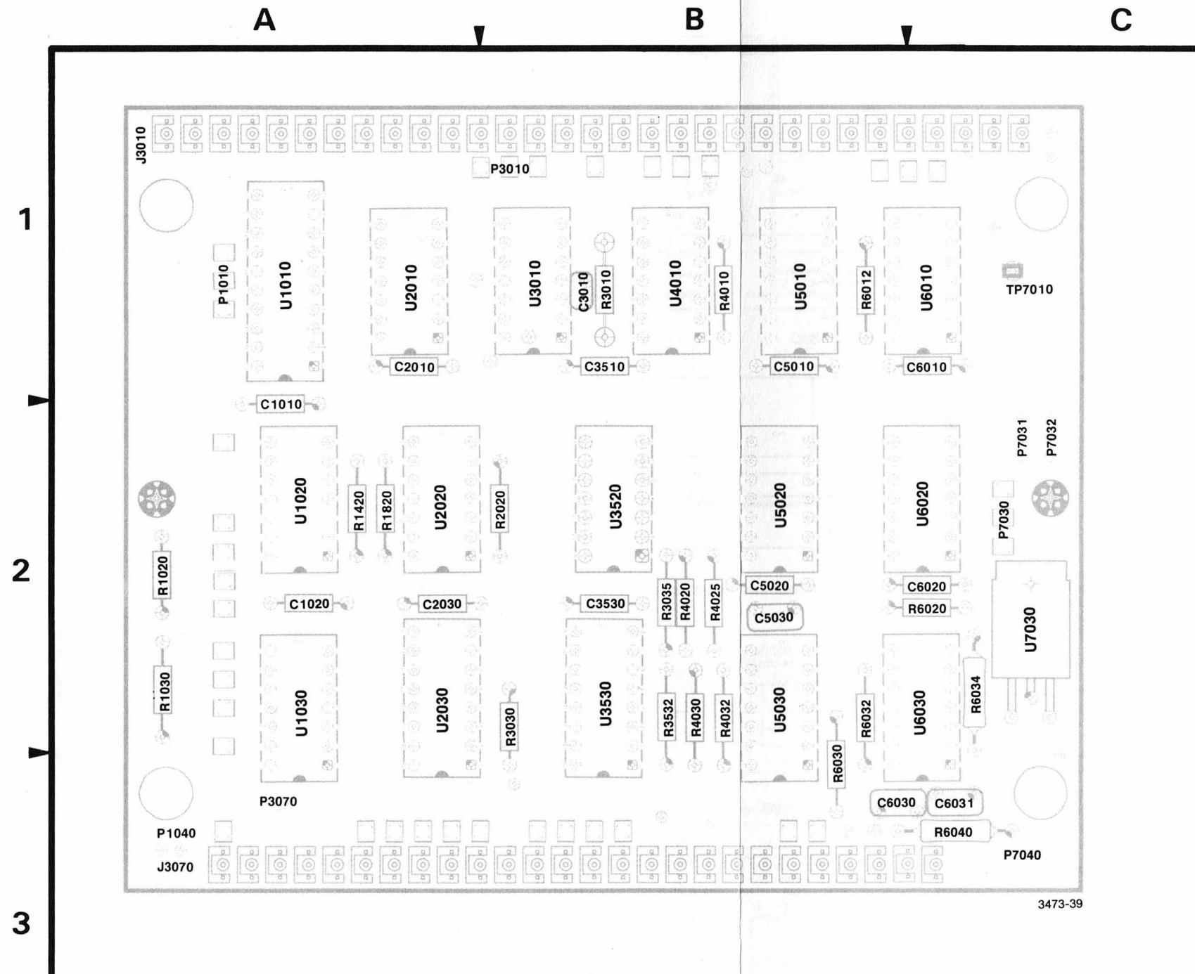
Figure 8-5. A2-Middle board component locations.
