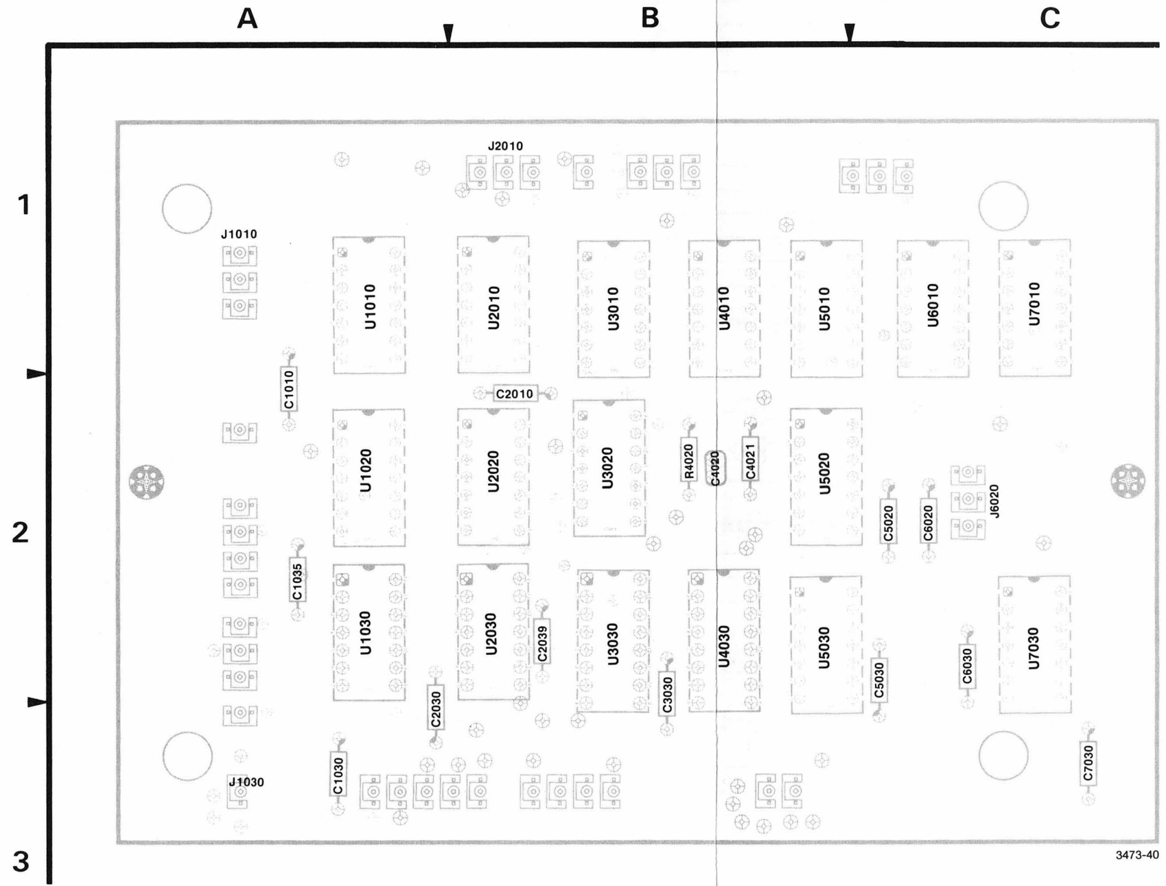
Figure 8-6. A3-Lower board component locations.
