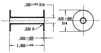
Note the wall thickness and ID tolerance of this part, demonstrating how parts can be made by electroforming which are very difficult or impossible to make any other way.
