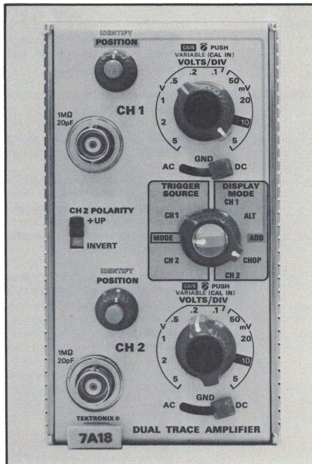
Fig. 2-1. Front-panel controls and connectors. (7A18 shown.)
