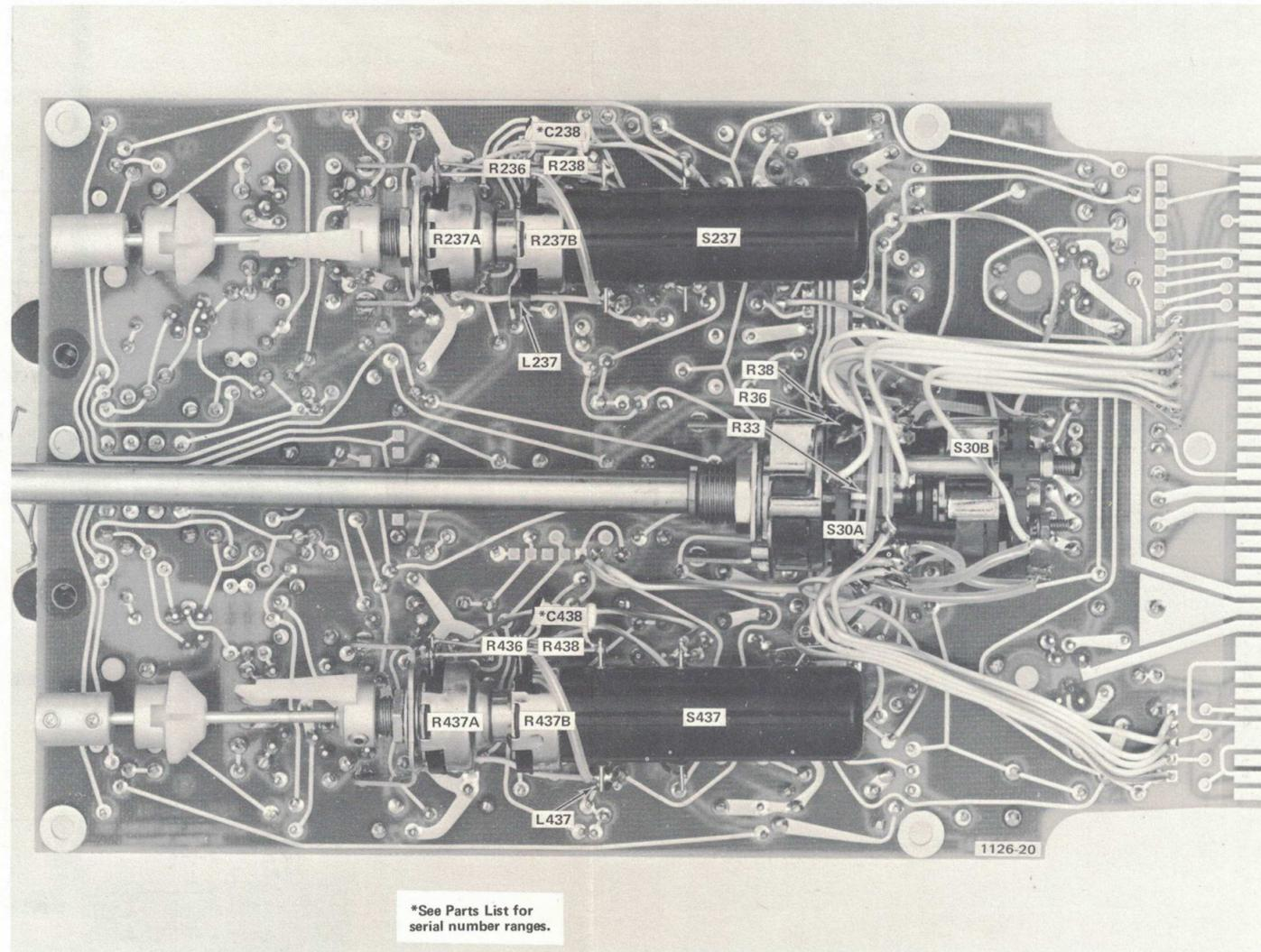
Fig. 7-2. A2 Amplifier Circuit Board Assembly (back view).
