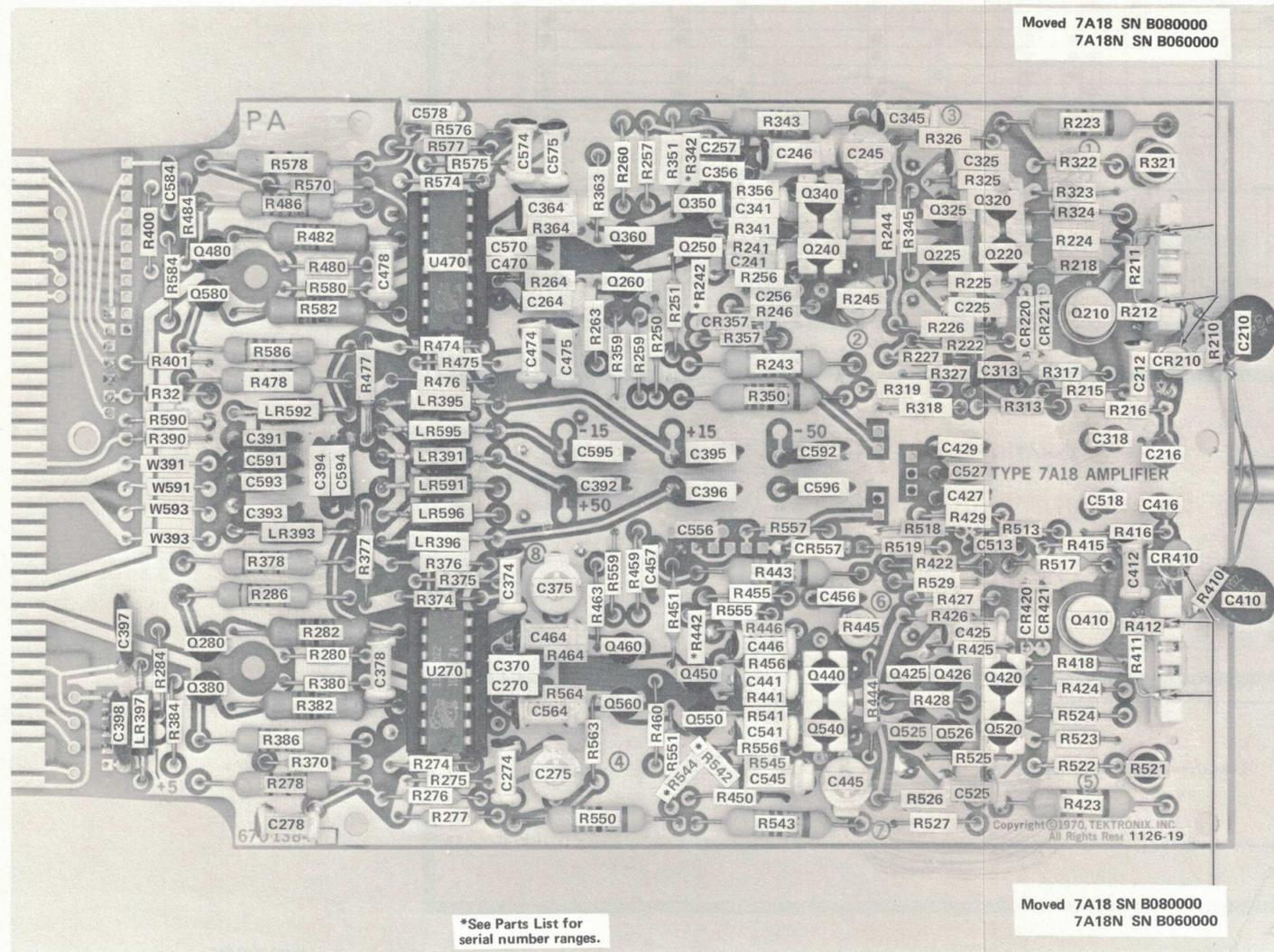
Fig. 7-1. A2 Amplifier Circuit Board Assembly (front view).
