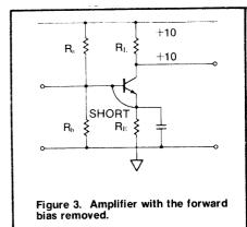
junction is reverse biased. The reverse biased diodes should be off, but because we have never been able to make a perfect diode, there is a very small current leaking across it. This leakage current flows through the collector-base junction and part of it goes through the base-emitter (control point) junction.
