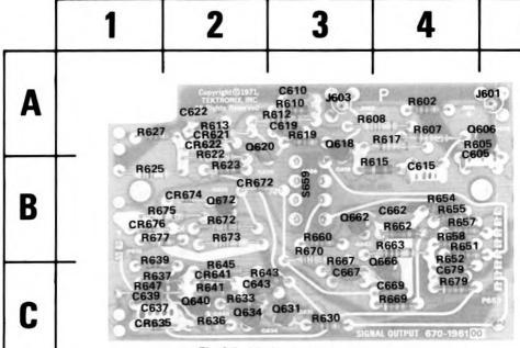
Fig. 6-7. A7 Output Signals circuit board.
