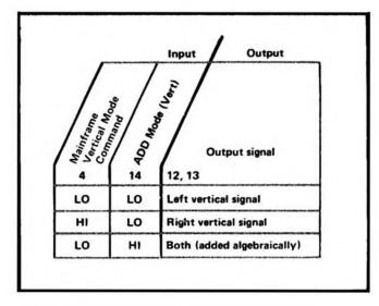
Fig. 3-17. Input/output table for Vertical Channel Switch.
