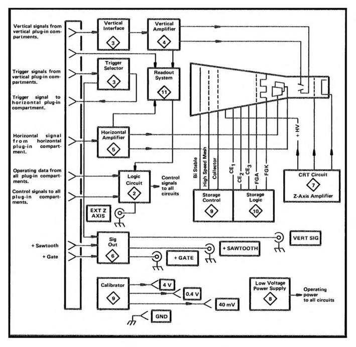
Fig. 3-1. Basic block diagram of 7623 Oscilloscope.
