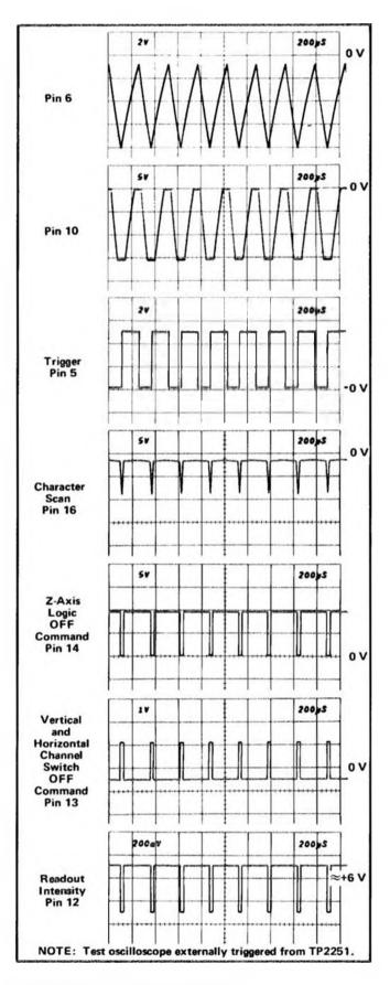
Fig. 3-28. Output waveforms of Timing stage.
