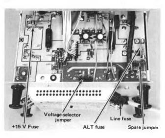
Fig. 1-1. Location of Voltage-selector jumper, spare jumper, and 230 V fuse in power-unit (shown removed).
