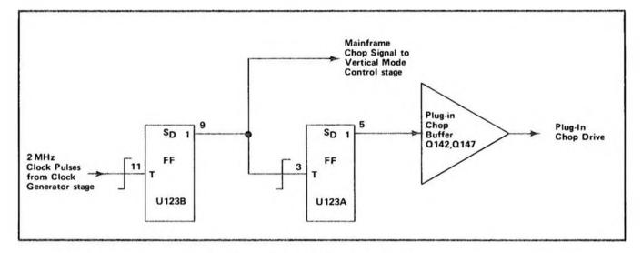
Fig. 3-7. Detailed logic diagram of Chop Counter stage.
