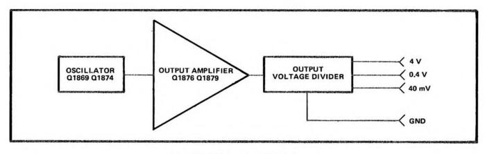
Fig. 3-20. Calibrator detailed block diagram.
