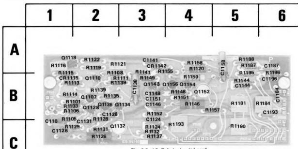
Fig. 6-8. A8 Z Axis circuit board.
