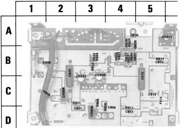
Fig. 6-11, A12 Rectifier circuit board.
