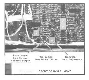
Fig. 2-8. Location of Calibrator adjustments (Cal-Storage board).
