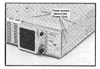
Fig. 4-1. Power Unit removal for the R7623.
