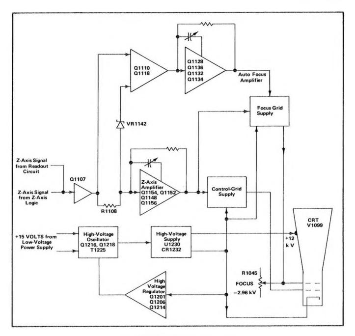
Fig. 3-21. CRT Circuit detailed block diagram.
