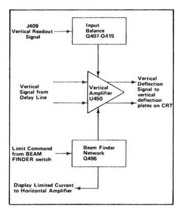
Fig. 3-18. Vertical Amplifier detailed block diagram.
