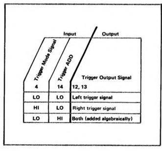
Fig. 3-15. Input/output table for Trigger Channel Switch stage.
