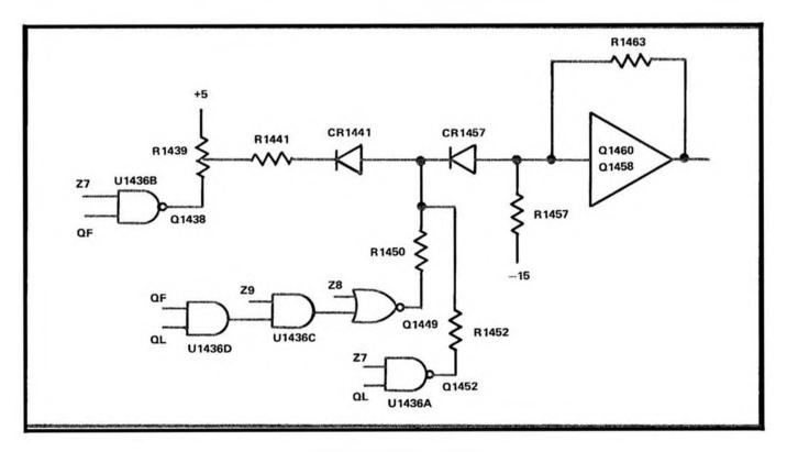
Fig. 3-43. Basic Collector Circuit.
