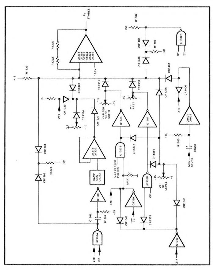
Fig. 3-44. Basic Bi-Stable Mesh Circuit.
