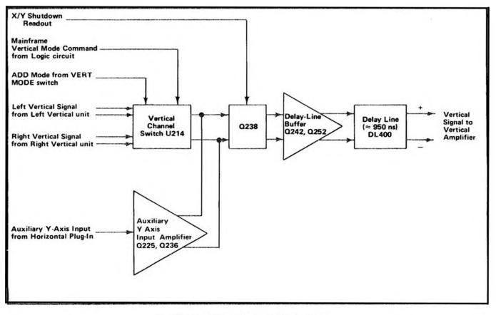
Fig. 3-16. Vertical Interface detailed block diagram.
