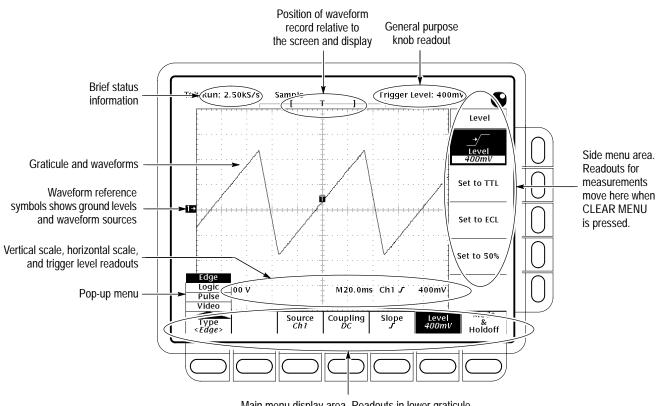
Main menu display area. Readouts in lower graticule area move here when CLEAR MENU is pressed.
