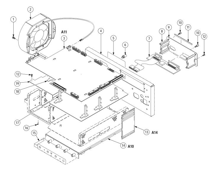
Figure 10–2: Outer-Chassis Modules
