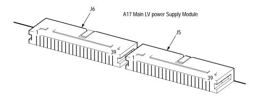
Figure 6–29: Power supply voltage measurement locations
