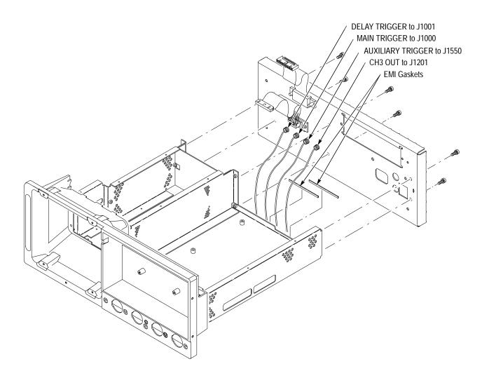
Figure 6–20: Rear Chassis Removal
