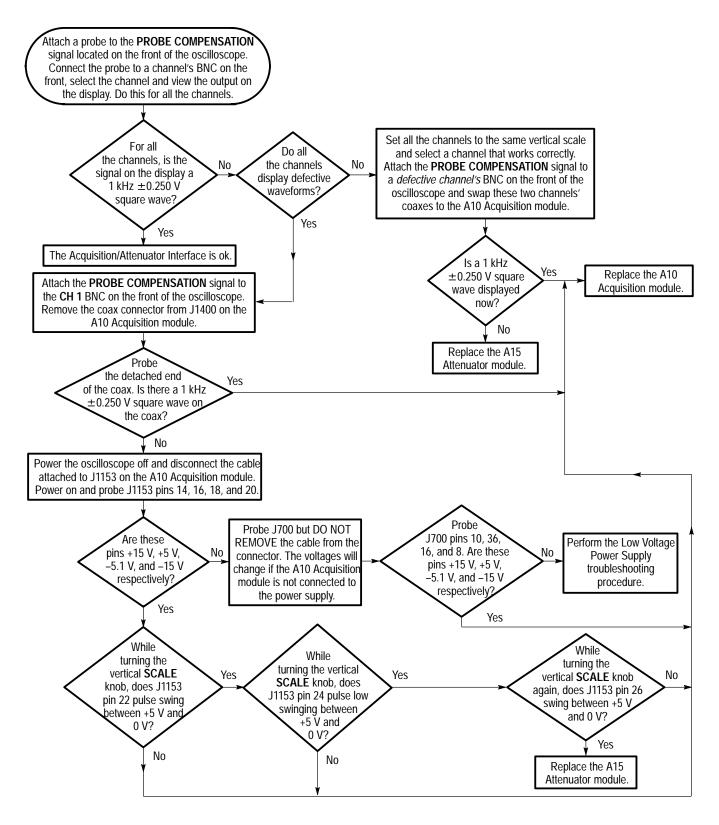
Figure 6–35: Attenuator/acquisition troubleshooting procedure
