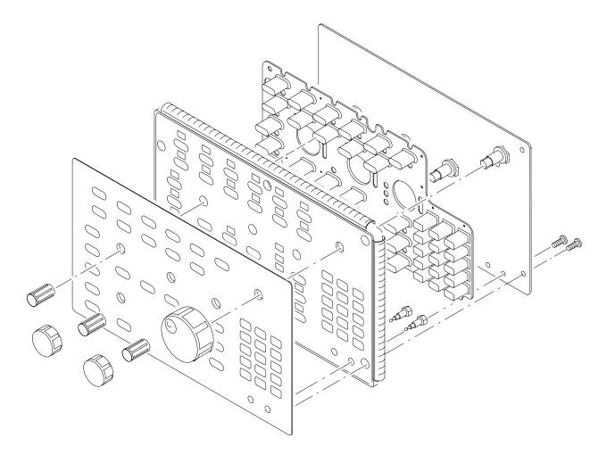
Figure 6–9: Disassembly of Front-Panel Assembly
