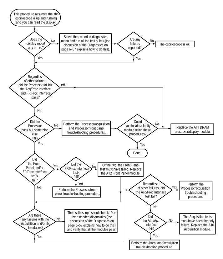
Figure 6–27: Module isolation troubleshooting procedure
