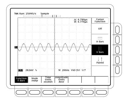
Figure 4–37: Line Count Accuracy Correct Result Waveform
