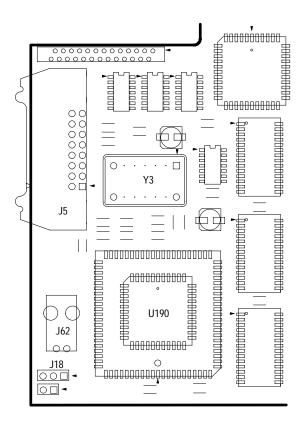
Figure 6–38: A11 DRAM processor/display Module (View of Lower Left Corner)
