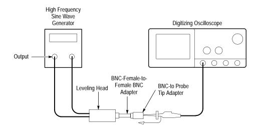
Figure 5–6: Initial Test Hookup
