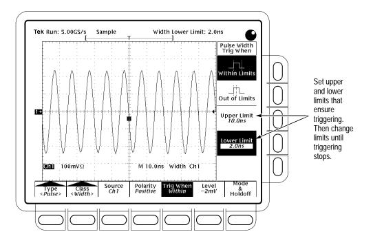
Figure 4–15: Measurement of Time Accuracy for Pulse and Glitch Triggering
