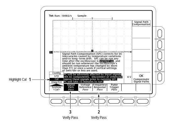
Figure 4–2: Verifying Adjustments and Signal-Path Compensation
