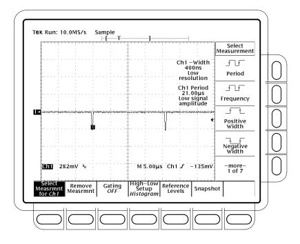
Figure 4–40: Sync Duty Cycle Test: Critically Adjusted Pulse
