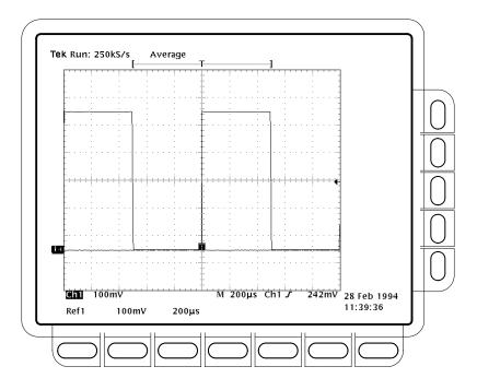
Figure 4–25: Measurement of Probe Compensator Amplitude
