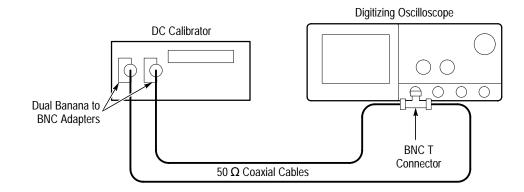
Figure 4–16: Initial Test Hookup
