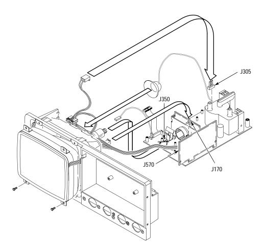
Figure 6–22: Display Assembly Removal
