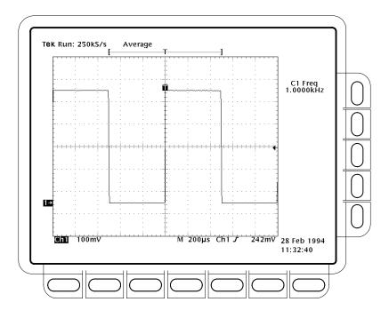
Figure 4–23: Measurement of Probe Compensator Frequency
