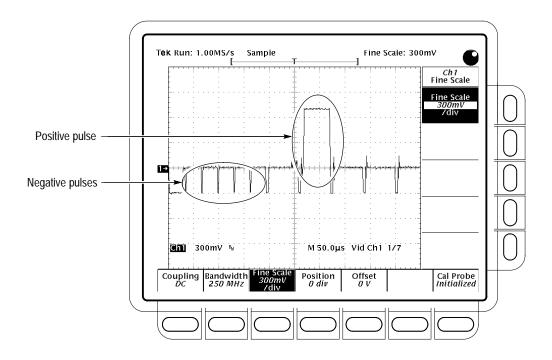
Figure 4–29: Triggered Signal Range Test – 300 mV
