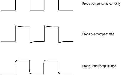
Figure 5-4: Proper and Improper Probe Compensation
