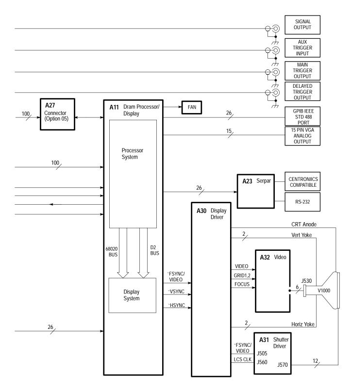
Figure 9–2: Block Diagram (Cont.)
