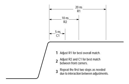
Figure 5–10: Adjustments versus Front-Corner Response
