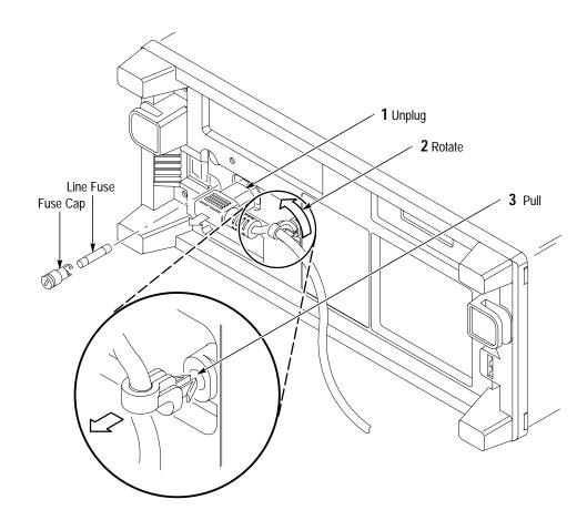
5. *Reinstallation:* Do in reverse steps 3 and 4 to reinstall the line cord and then the line fuse.
