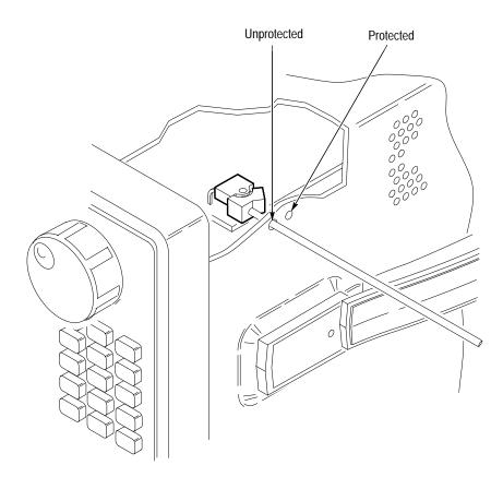
Figure 6–25: Accessing the protection switch
