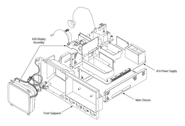
Figure 6–3: Inner-Chassis Modules
