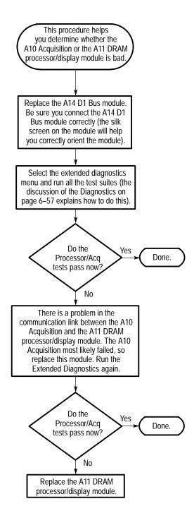
Figure 6–33: Processor/acquisition troubleshooting procedure
