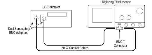
the other side of the BNC T connector. Now connect the BNC T connector to **CH 1**. See Figure 4–24.
