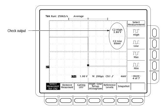
Figure 4–21: Measurement of Main Trigger Out Limits
