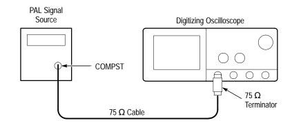
Figure 4–26: Jitter Test Hookup
