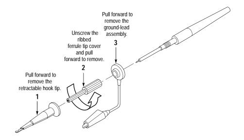
Figure 5–5: Exposing the Inner Probe Tip
