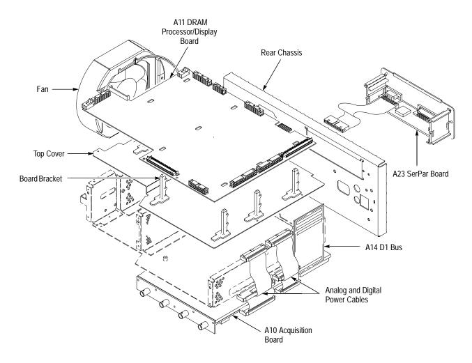
Figure 6–2: Outer-Chassis Modules
