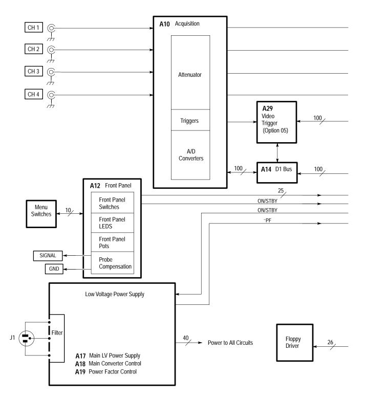
Figure 9–2: Block Diagram
