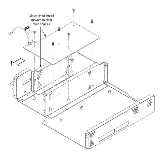
Figure 6–23: Display Driver Board Removal
