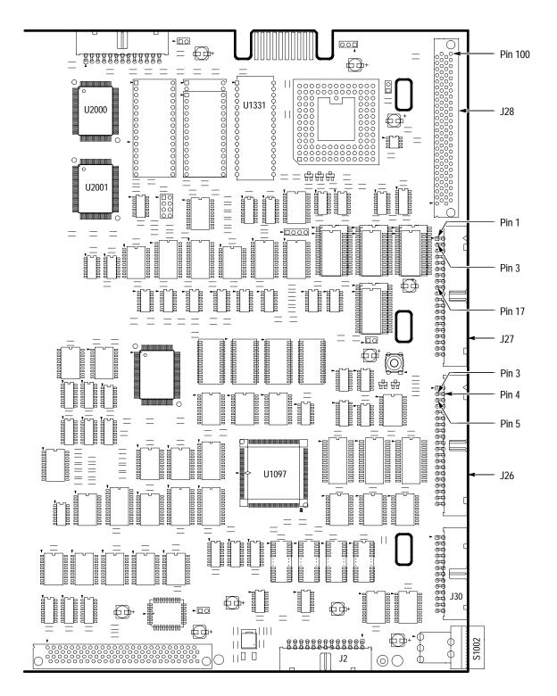
Figure 6-36: A11 DRAM processor/display module
