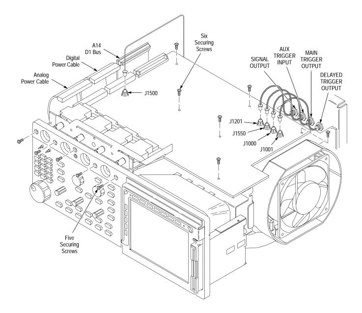
Figure 6–18: A10 Acquisition Board Removal
