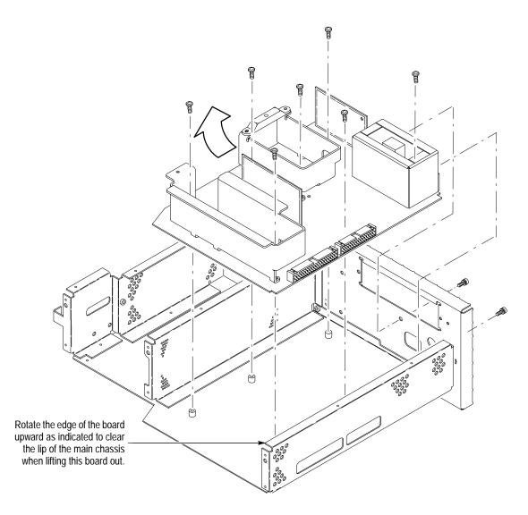
Figure 6–21: A16 Low Voltage Power Supply Removal
