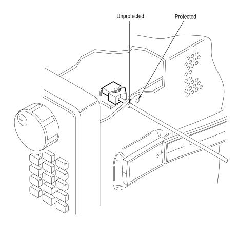
Figure 5–1: Accessing the Protection Switch
