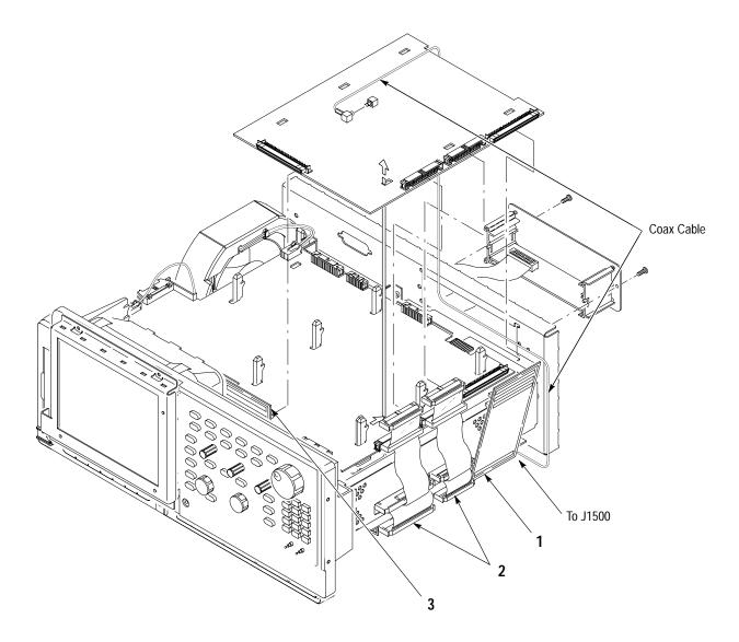
Figure 6–15: Circuit Board Removal
