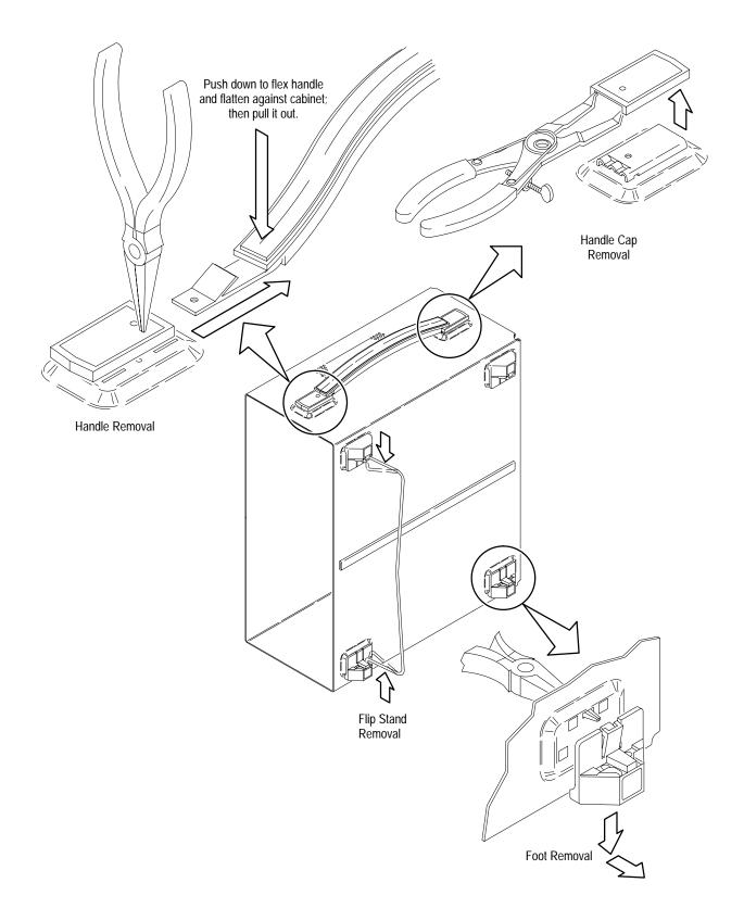
Figure 6–10: Cabinet Modules Removal
