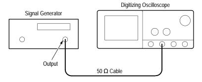
Figure 4–31: 60 Hz Rejection Test Hookup
