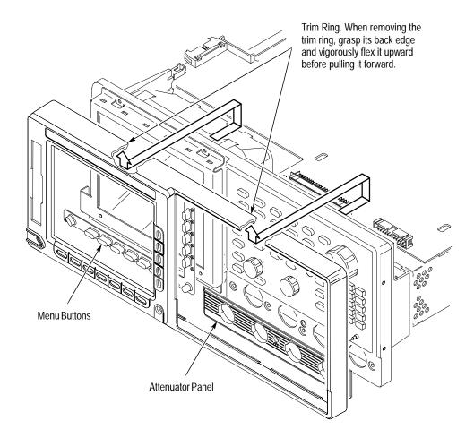
Figure 6–7: Front Cover, Trim Ring, Menu Buttons, and Attenuator Panel Removal (Front Cover not Shown)
