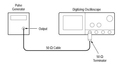
Figure 4–38: Setup for Sync Duty Cycle Test
