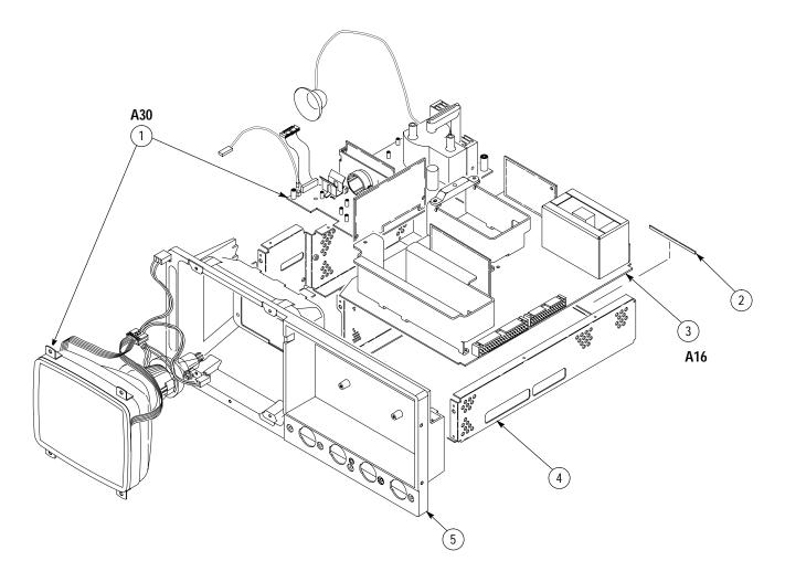
Figure 10–3: Inner-Chassis Modules
