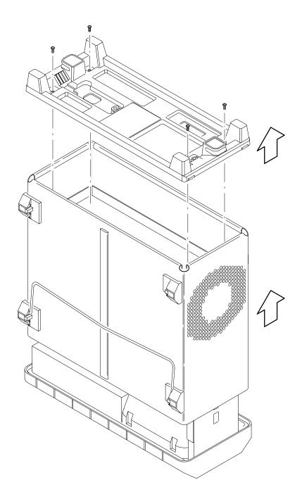
Figure 6–6: Rear Cover and Cabinet Removal
