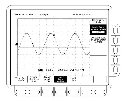
Figure 4–32: 60 Hz Rejection Test Setup Signal
