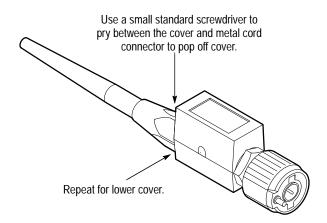
Figure 5–7: Exposing the Probe Body
