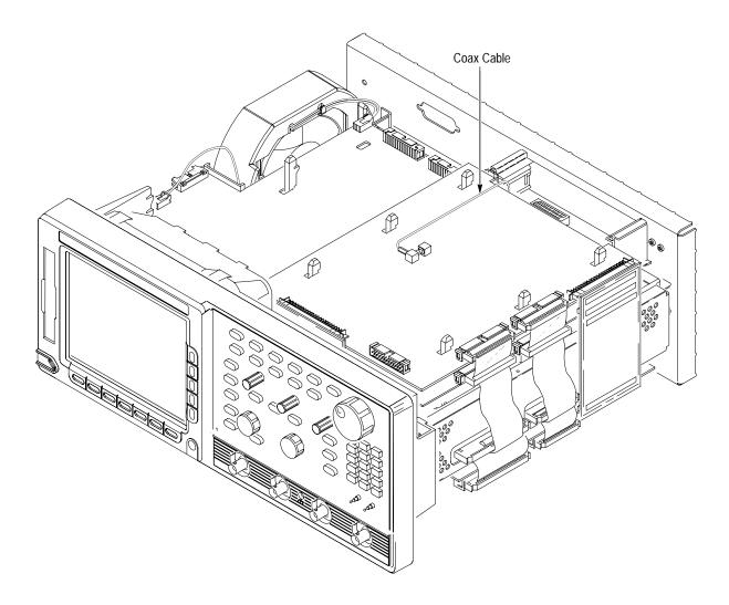
Figure 6–14: Circuit Board Installed
