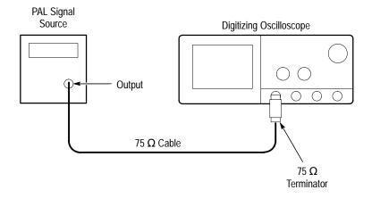
Figure 4–35: Line Count Accuracy Test Hookup
