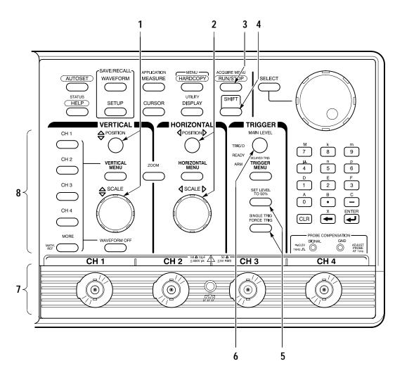
**2.** Select the waveform source(s). Position, scale, and set trigger level for waveform source(s) directly from the front panel. The steps that follow provide examples of possible control selections.
