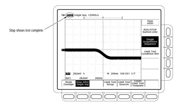
Figure 4–28: Jitter Test When Completed – TDS 684B Shown
