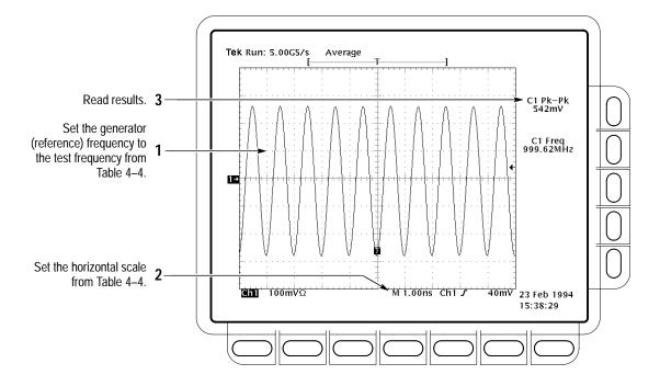
Figure 4–9: Measurement of Analog Bandwidth
