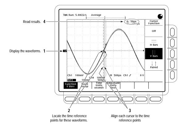
Figure 4–11: Measurement of Channel Delay – TDS 684B Shown
