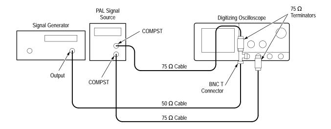
Figure 4–33: Subsequent 60 Hz Rejection Test Hookup
