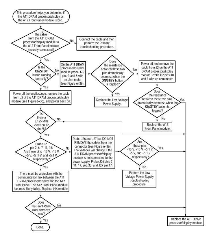
Figure 6-34: Processor/front panel troubleshooting procedure
