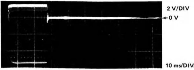
F.) At TP1958 H.V. Current Sens during sampling period with short on -2950 supply.
