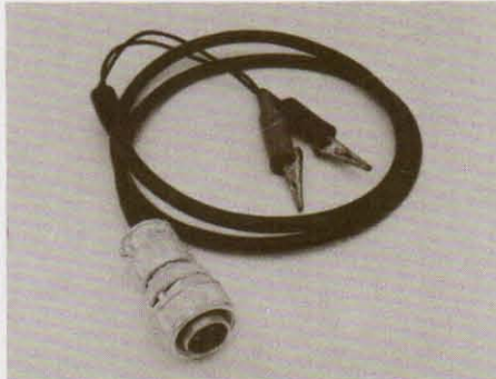
Model 1506 Input Cable: 1.2m (4 ft.) triaxial cable with a low thermal mating connector to Model 181 on one end and two copper alligator clips on the other.
