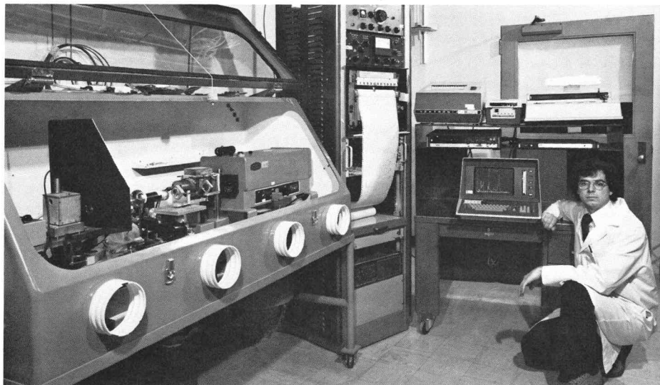
Fig. 2. Microscope spectrophotometer and Tektronix 4051 system.
