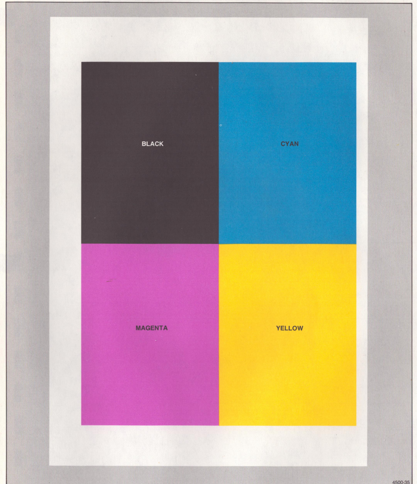
Figure 13-8. 4-Solid/TV Test Pattern (TEST PATTERN SELECT #3).
