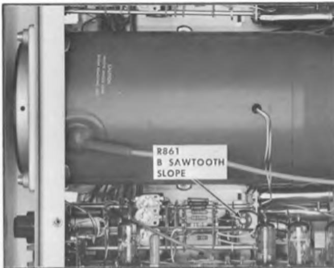
Fig. 6-35. Adjustment location for B sweep sawtooth slope.
