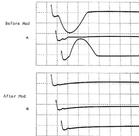
Figure 1. A—Waveform aberration before addition of R1020. B—After addition. Signal Source: 1 Volt Cal, Sweep Rate 1  $\mu$ s/cm. Type W Unit Control Settings:  $V_c + 11$ , INPUT ATTEN 1, DISPLAY A- $V_c$ , MILLIVOLTS/CM 5. (Triple exposure photos.)
