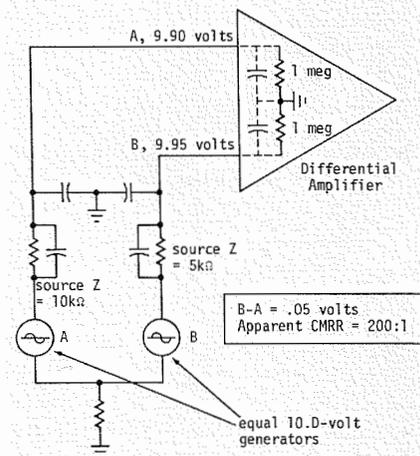
Figure 7. Schematic that shows the relationship of test-point source impedance to the amplifier-input impedance, and also shows the apparent CMRR caused by large value difference between test-point impedances.
