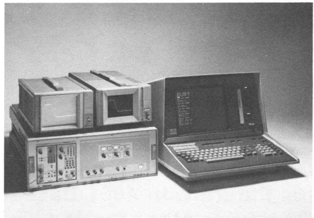
The Tektronix 7912AD Programmable Digitizer with its 7A16P Programmable Amplifier and 7B90P Programmable Time Base plug-ins (lefthand side of front panel) operates under program control from the 4051. Sitting on top of the 7912AD, an XYZ monitor and a TV monitor display the digitized waveform in 7912AD data memory.
