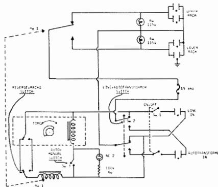
Figure 2 shows the circuit design used in this cycling unit. Notice the 15 amp fuse in the common supply to the upper and lower racks. This fuse prevents excessive current drain in the event of short circuits in the unit or the instruments under-going cycling.
