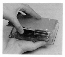
B. Disassembling the tape cartridge.
