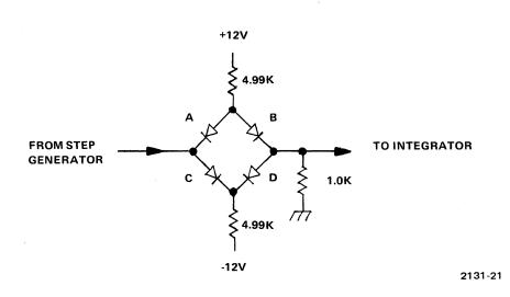
Fig. 5-6. Diode Bridge Functioning as a Current Switch.
