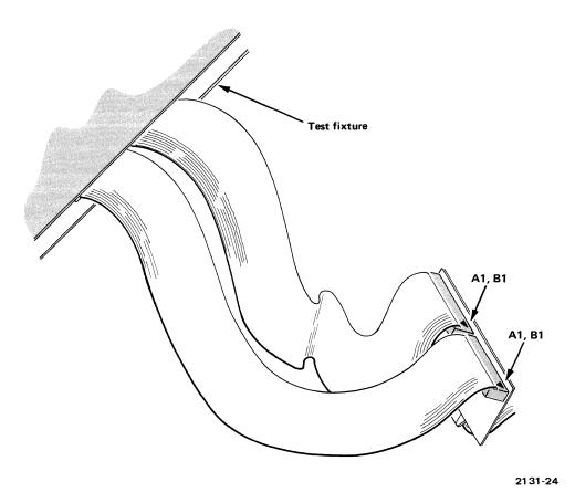
Fig. 6-3. Test Board Buffer Adapter Cable Connections.
