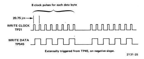
Fig. 6-6. Write waveforms.
