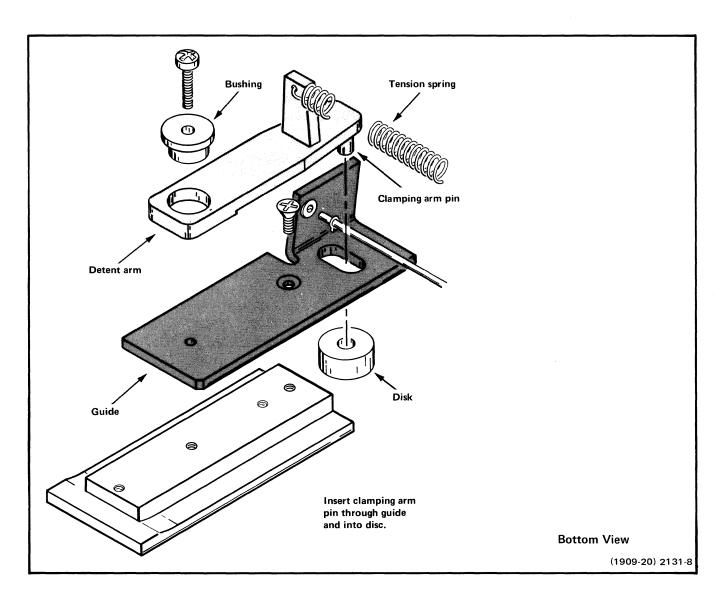
Fig. 3-11. Cartridge Guide Components.
