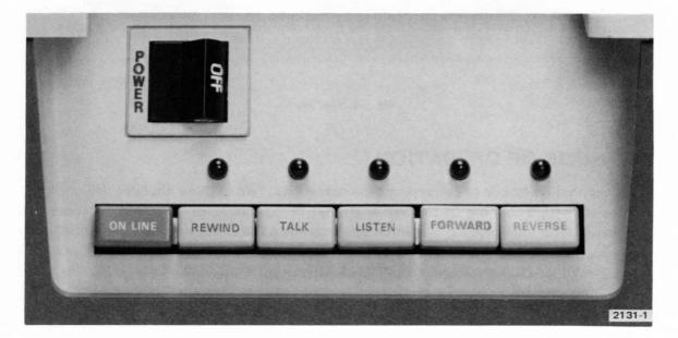
Fig. 1-2. Front Panel Switches and Indicators.
