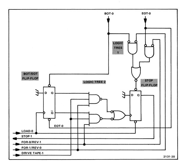
BOT was sensed, reverse for EOT), Logic Tree 2 clocks the STOP Flip-Flop, removing the STOP signal. The Stop Tape Control may also be reset by a LOAD pulse.
