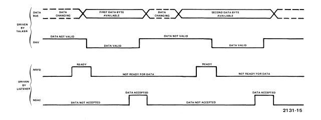
Fig. 4-2. GPIB Transfer Bus Handshake Sequence.
