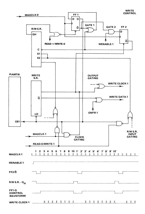
Fig. 5-7. Write Control Circuitry and Waveforms.
