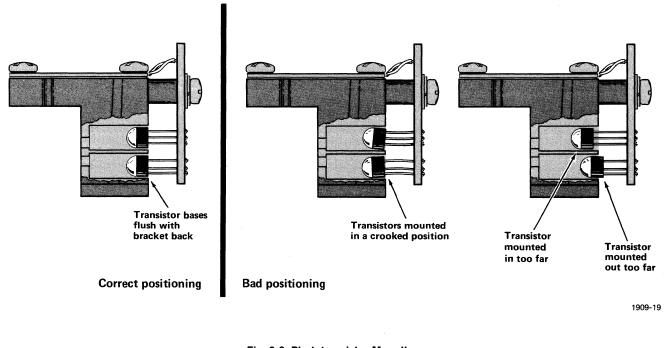
Fig. 3-9. Phototransistor Mounting.
