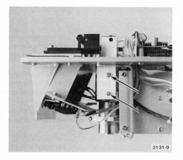
Fig. 3-12. Head Bracket Mounting Screws.
