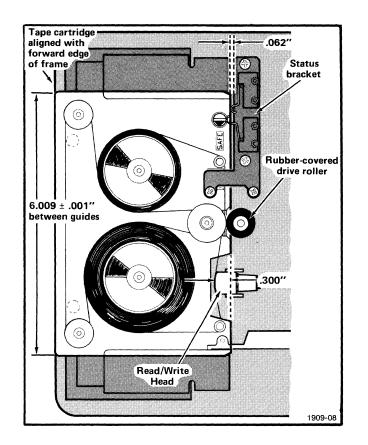
Fig. 2-4. Cartridge Position Dimensions.
