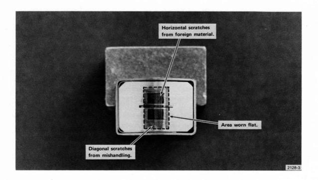
Fig. 3-2. Tape Head Damage.
