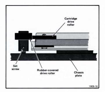
Fig. 3-6. Rubber Roller/Cartridge Roller Positioning.
