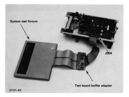
Fig. 6-1. System Test Fixture and Test Board Buffer Adapter.
