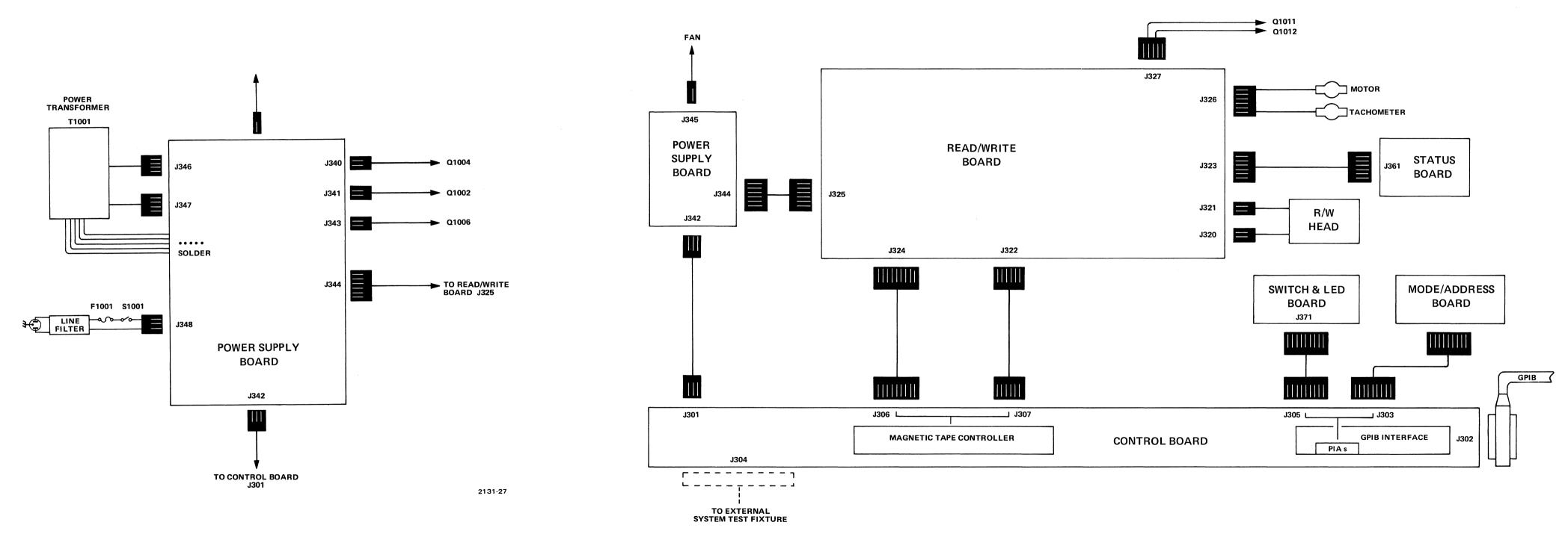
Fig. 8-2. Power Supply Board Interconnection Diagram.
