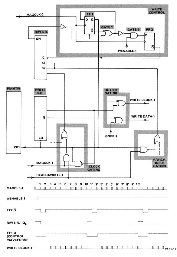
Fig. 5-2. Write Control Circuitry and Waveforms.
