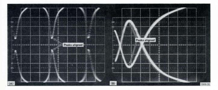
Fig. 3-18. Correct Skew Adjustment Waveforms.
