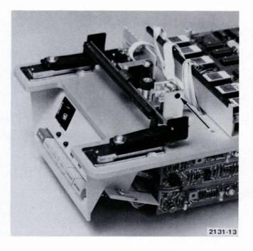
Fig. 3-19. Skew (Azimuth) Adjusting Screw.
