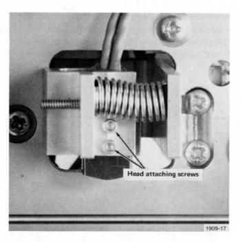
Fig. 3-7. Location of Head Attaching Screws.
