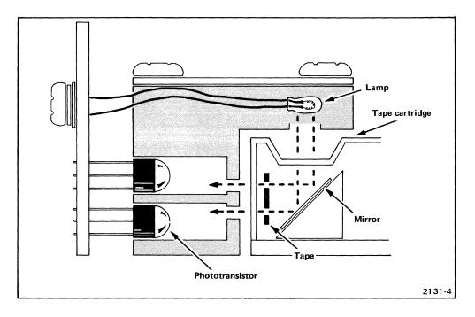
Fig. 2-3. Position Marker Sensing.
