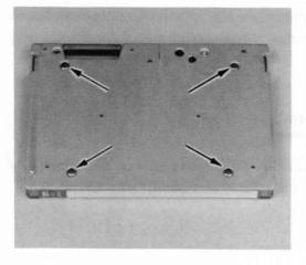
A. Cartridge attaching screws.
