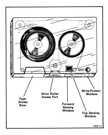
Fig. 2-2. Tape Cartridge Parts.
