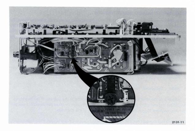
Fig. 3-16. +12 Volt Supply Adjustment Locations.
