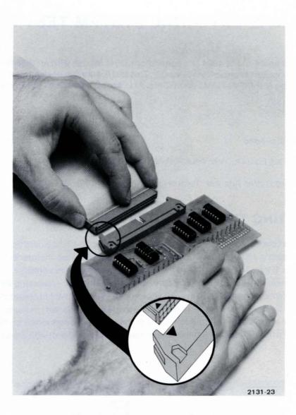
Fig. 6-2. Connector Alignment.
