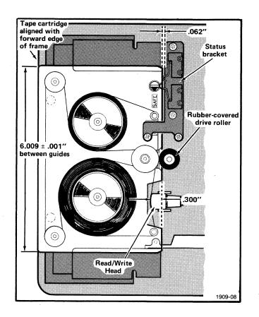
Fig. 3-10. Cartridge Position Dimensions.
