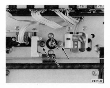
Fig. 3-4. Motor Attaching Screws.
