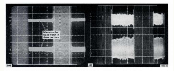
Fig. 3-20. Correct Height Adjustment Waveforms.
