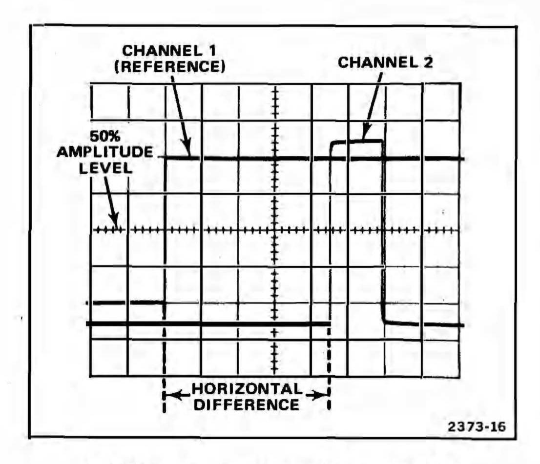
Fig. 16. Measuring time difference between two pulses.
