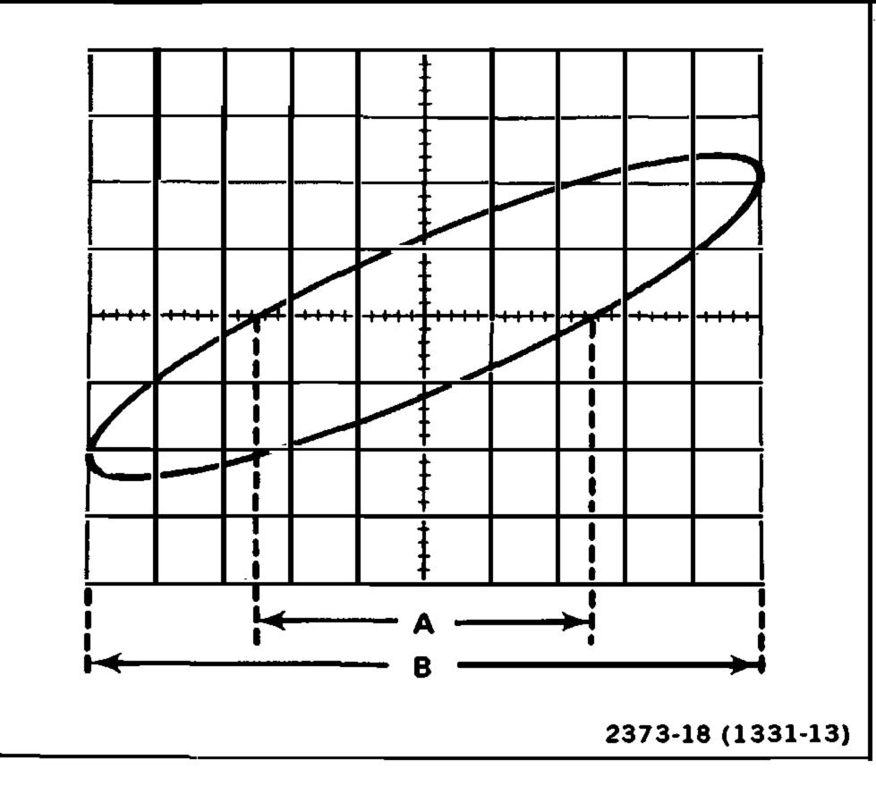
Fig. 18. Phase difference measurement from an X-Y display.
