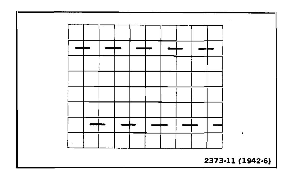
Fig. 11. Display of .5V PROBE ADJ output signal.
