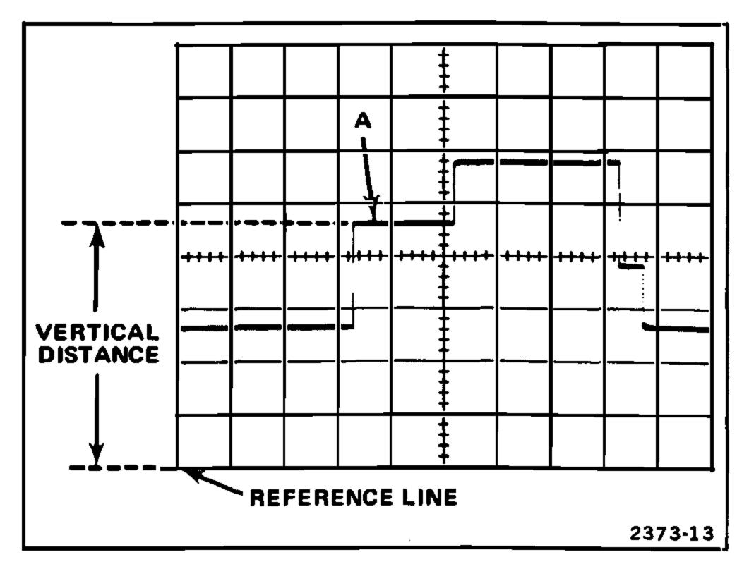
Fig. 13. Measuring instantaneous dc voltage with respect to a reference voltage.
