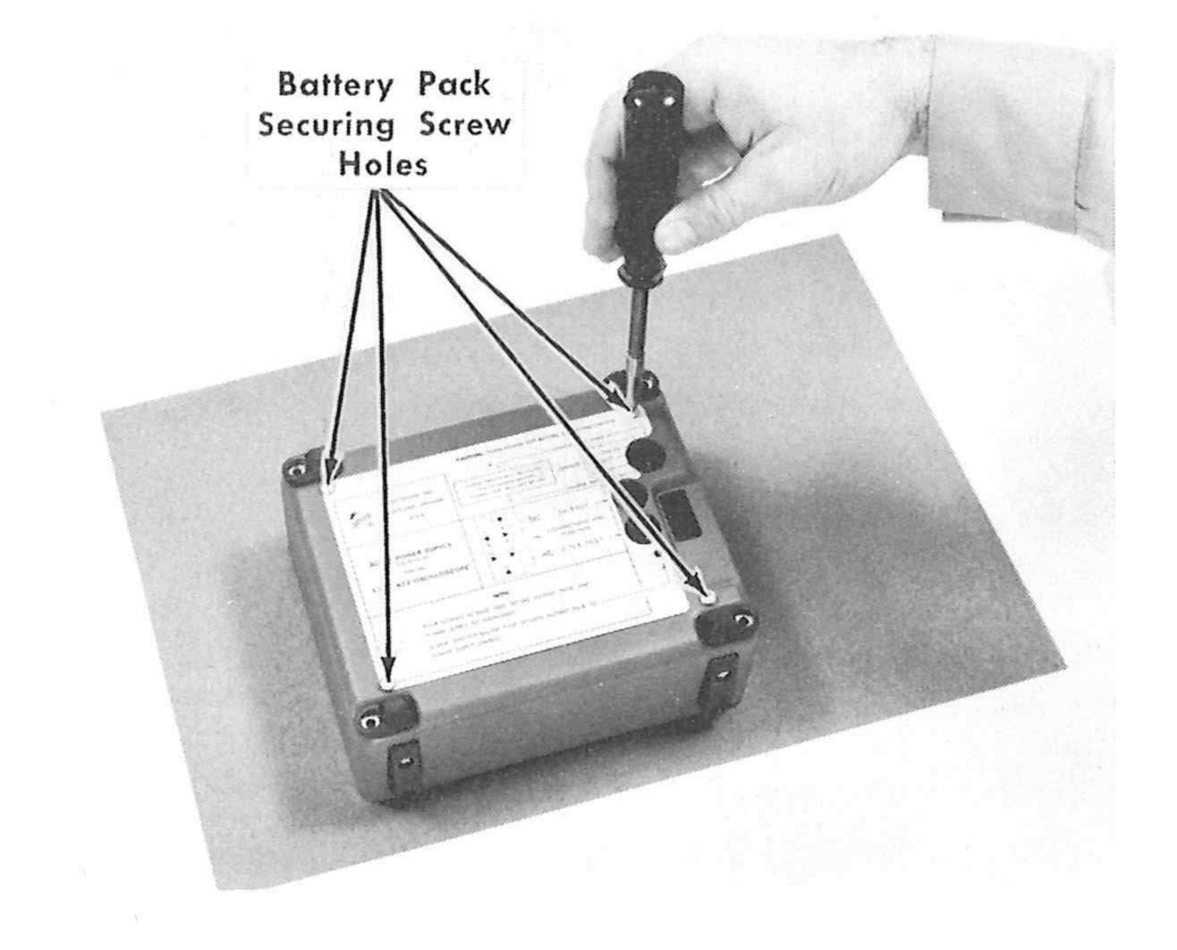
e. Start each of the four long screws, removed from the Battery Pack in step 2b into the four holes indicated, then tighten the four screws securely.
