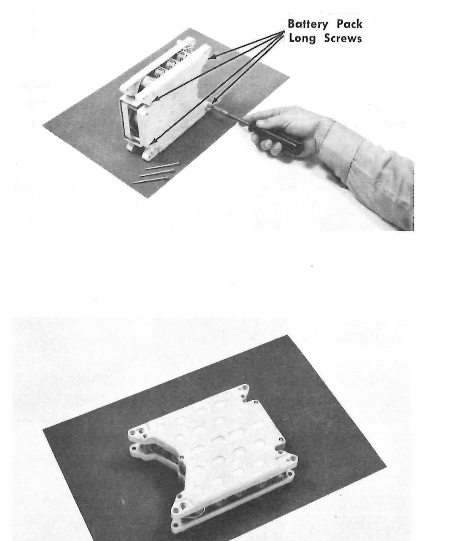
c. Set the Battery Pack on a non-conducting flat sur-face so it is resting on its interconnecting banana jacks and spring bracket.
