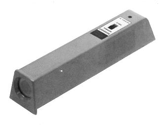
The J6502-2 is designed to measure irradiance in  $mw/m^2$  where light incident upon a surface must be measured. Measurements are made with the J6502-2 pointed at the light source. Narrow angle light sources such as lasers which do not fill the entire active area of the sensor may be measured in which case  $1mW/m^2$  =  $1 \times 10^{-4} mW$ .
