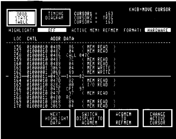
Figure 4. HARDWARE format shows instruction mnemonics.
