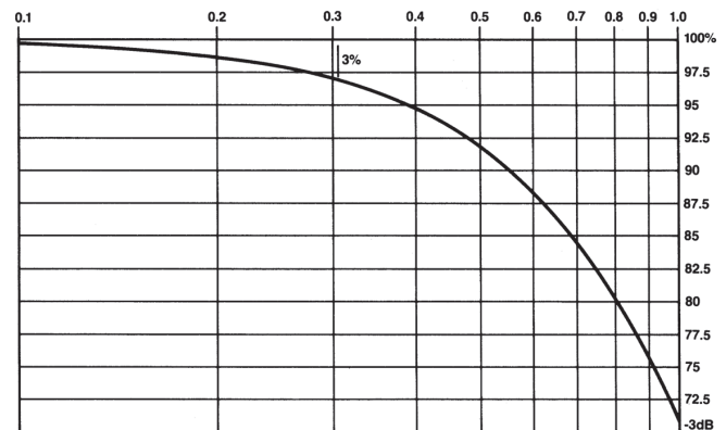
Figure 4.8. Bandwidth derating curve.
