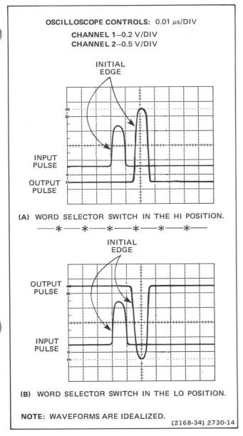
Figure 4-4. Test oscilloscope displays for Minimum Input Swing, Pulse Width, and Propagation Delay Check.
