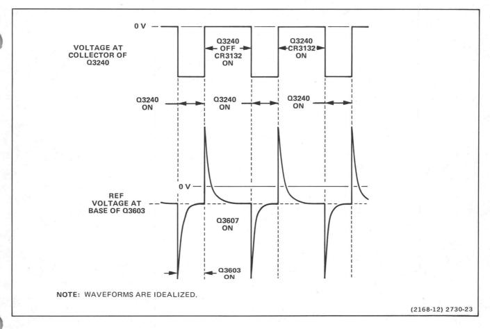
Figure 3-8. -5-Volt Supply timing diagram.
