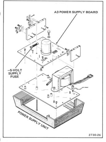
Figure 5-6. Power Supply unit circuit board location.
