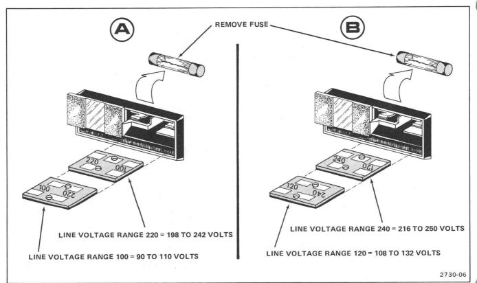
Figure 2-1. Line Voltage Selector card positioning.
