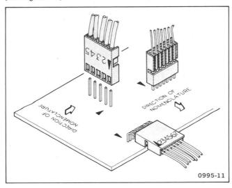
Figure 5-4. Multi-conductor holder orientation.
