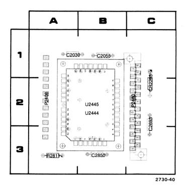
Figure 8-3. Data Input circuit board component locations.
