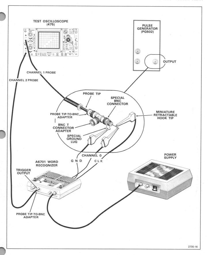
Figure 4-5. Minimum Setup and Hold and Clock Period Check test setup.
