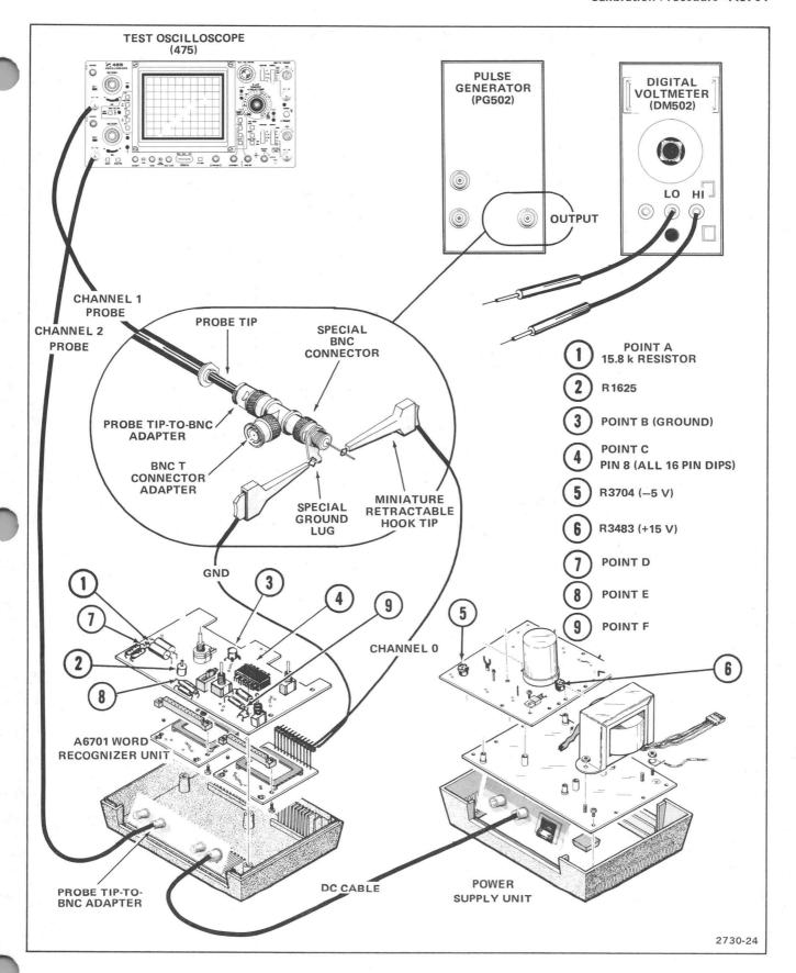
Figure 4-7. System adjustments setup and test points.
