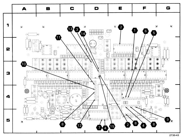
Figure 8-2. Waveform test point locations.
