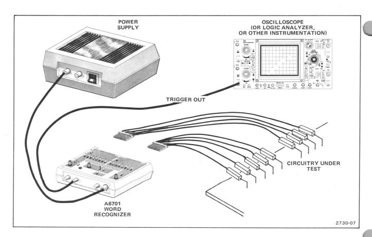
Figure 2-5. Operation setup (18-channel system).
