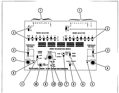
Figure 1, Partial WR controls (TRIGGER STATUS SWITCH changes).
