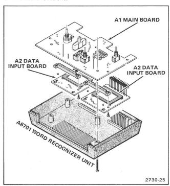
Figure 5-5. Word Recognizer unit circuit board locations.
