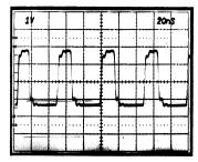
(Seen at probe tip-to-bnc adapter.)
