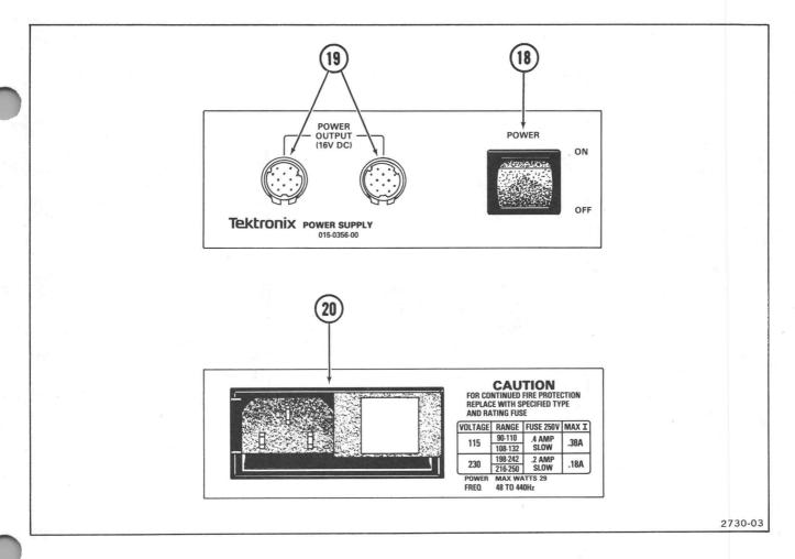
Figure 2-4. Power Supply controls and connectors.
