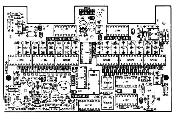
Figure 3. Al Main circuit board component location changes.
