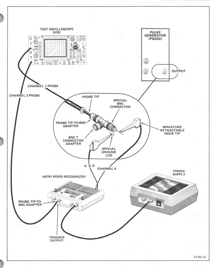
Figure 4-3. Minimum Input Swing, Pulse Width, and Propagation Delay Check test setup.
