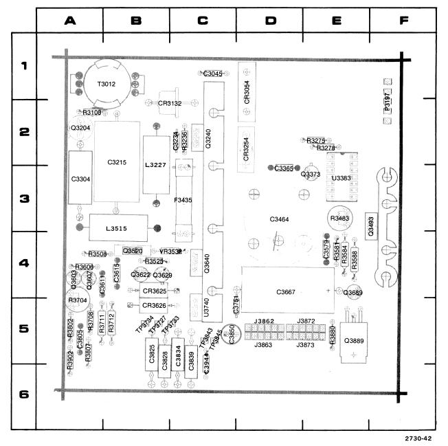
Figure 8-5. Power Supply circuit board component locations.
