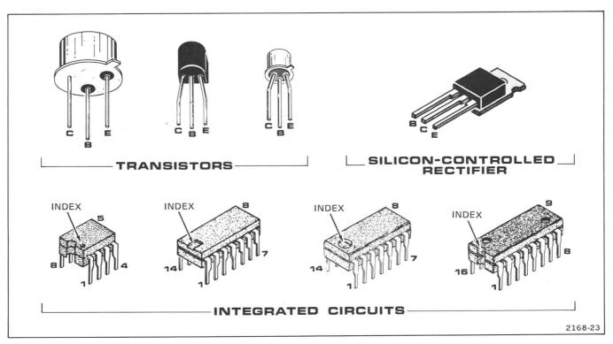
Figure 5-3. Lead configuration for semiconductor devices.
