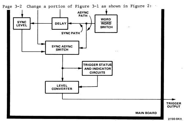
Figure 2. Partial block diagram (Trigger changes).
