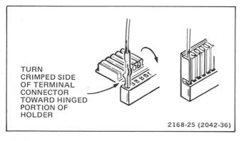
Figure 5-7. Pin connector replacement.
