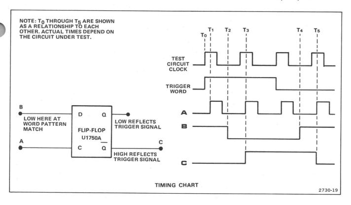
Figure 3-5. Sync Level Flip-Flop circuit analysis.
