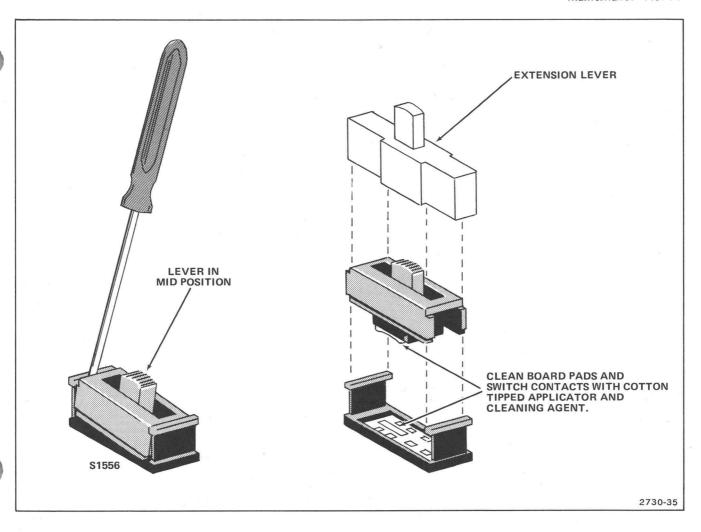
Figure 5-1. SYNC ASYNC switch cleaning.
