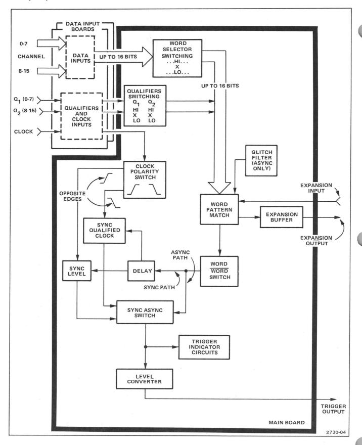
Figure 3-1. Block diagram.
