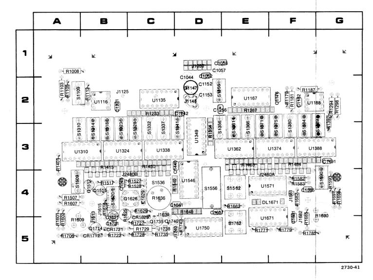
Figure 8-4. Main circuit board component locations.
