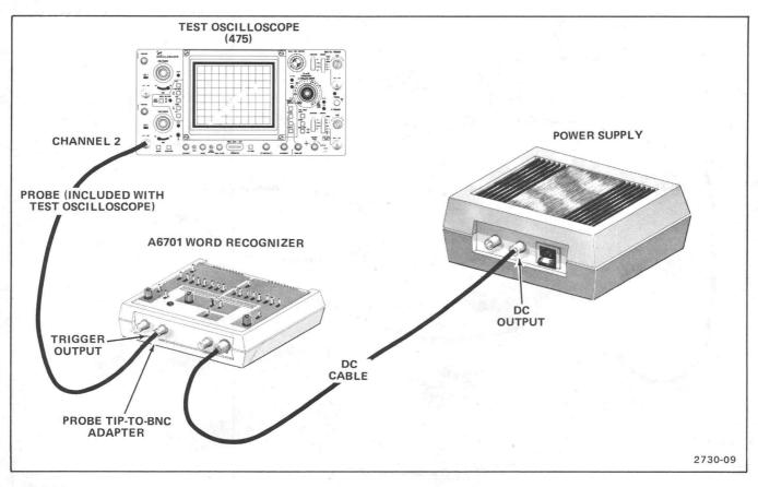
Figure 4-1. Trigger Indicator and Output Levels Check test setup.
