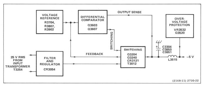
Figure 3-7. -5-Volt Supply block diagram.
