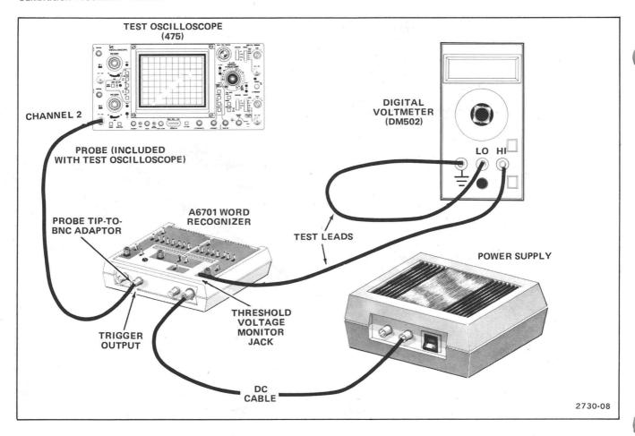
Figure 4-2. Threshold Levels Check test setup.
