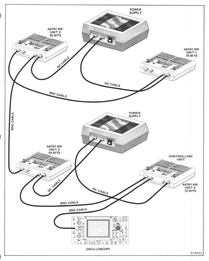
Figure 2-2. A6701 System configuration.
