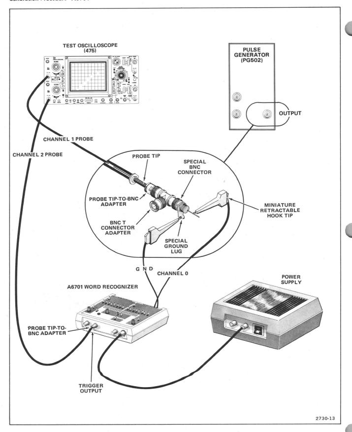
Figure 4-6. Glitch Filter Check test setup.
