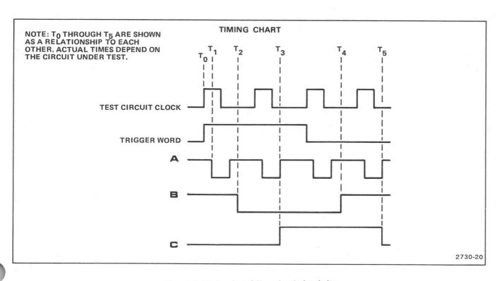
Figure 3-6. Timing chart, falling edge clock polarity.
