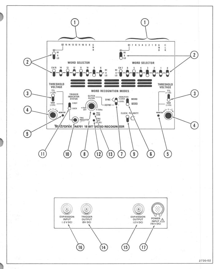
Figure 2-3. WR controls, connectors, and indicators.
