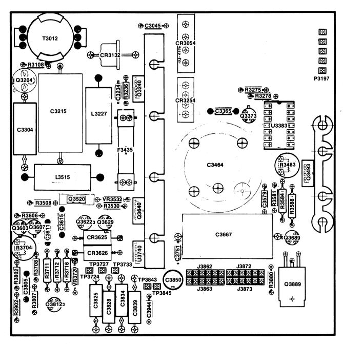
Figure 4. A3 Power Supply board component location changes.
