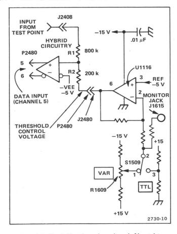
Figure 3-2. Threshold setting and one channel of input data.
