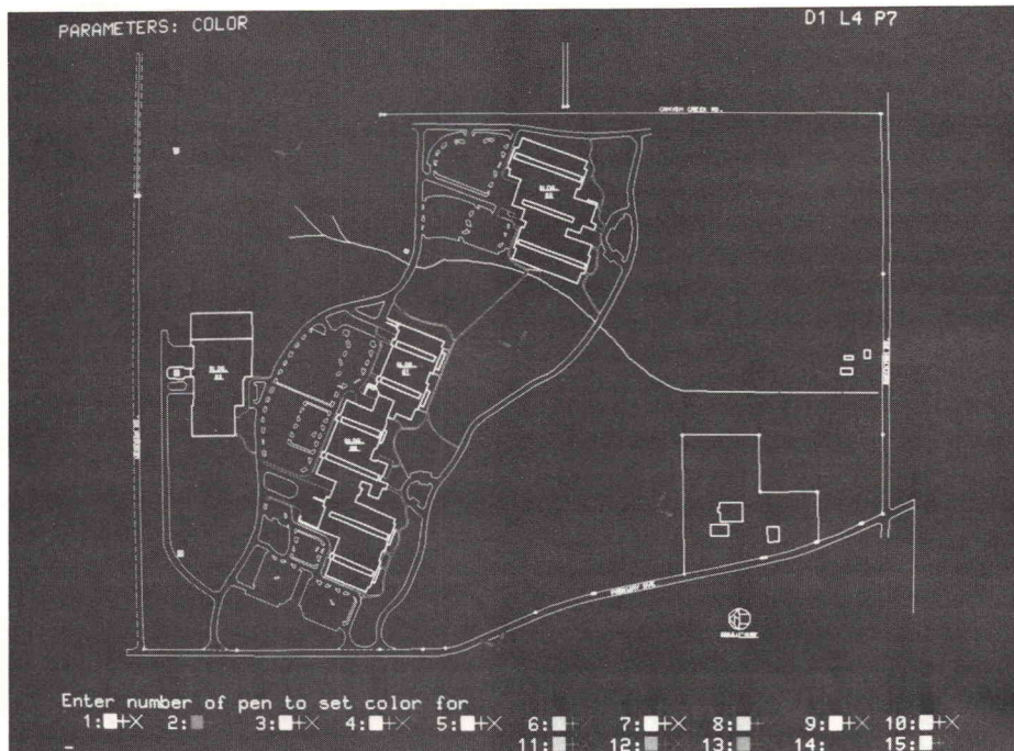
Figure 5. Irregular lines such as creeks and other waterways can be quickly scanned.
