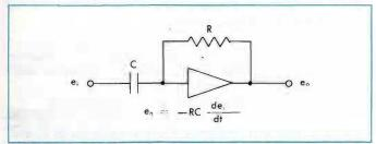
DIFFERENTIATION is accomplished by placing a capacitor in the input circuit. The unique characteristic of differentiation is its ability to extract higher frequency waveform components. It can advantageously detect minute information such as transients and slope changes. Differentiation of waveforms with significant components as high as 1.5 MHz is possible.
