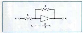
AMPLIFICATION is determined by the ratio of input to feedback resistors. This provides convenient signal step-up or step-down, with low output impedances, to over 750 kHz. Use of external compensation extends the closed-loop gain-bandwidth product to 10 MHz or more.
