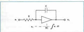
INTEGRATION is obtained by placing a capacitor in the feedback loop. Unlike the RC integrator, this circuitry permits loading of the output, and integration without loss of signal level. Integration at repetition rates of approximately 5 MHz is possible. Low-frequency rejection allows drift-free repetitive-waveform integration.
