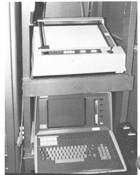
Inside the screen room, the data is fed to the Tektronix 4051 and printed on the 4662.
