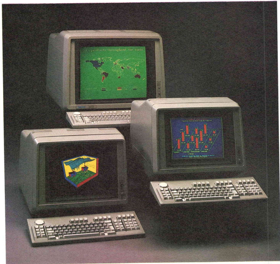
CX4106, CX4107 and CX4109 Computer Display Terminals offer direct coaxial connection to IBM 3270 controllers, giving IBM users access to the PLOT 10 graphics command set while retaining the IBM-style keyboard and alphanumeric capabilities.
