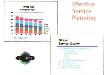
Figure 4. A presentation visual may include graph output from the GRAPH module, a bulleted list and extra free-form type from the TYPE module, and a special-purpose illustration from the DRAW module. Output from each TekniCAP module is directed to the appropriate area of the display using the VIEW module.
