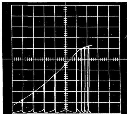
Figure 12. Transfer curve across zero bias.  $V_{GS}$  (horizontal) = 0.5 V/cm,  $I_{DSS}$  (vertical) = 2 mA/cm. Center vertical graticule line is zero bias. Negative bias to left, positive bias to right of center line. Crowding of markers on right hand side is due to gate drawing current.
