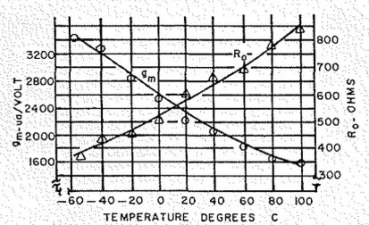
Figure 9. (a) Graph of saturation current under zero bias conditions and with the forward voltage from Drain-to-Source set at 50 volts. (b) Cross graph of  $g_m$  and output resistance plotted against temperature.
