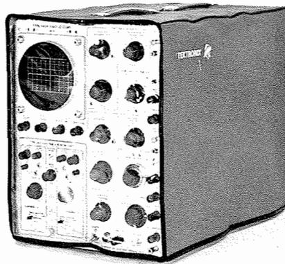
Figure 1. New dust cover for Tektronix oscilloscopes shown on a Type 545B Oscilloscope.
