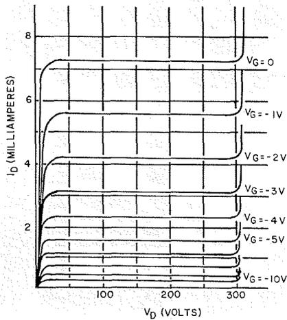
Figure 5. A chart of the  $V_D$  vs  $I_D$  curves of another FET showing Zener-knee breakdown of Gate-to-Drain back-biased diode. An extension of the curves shown in Figure 4 would reveal a similar tendency of this FET to avalanche at some certain  $V_D$  voltage.
