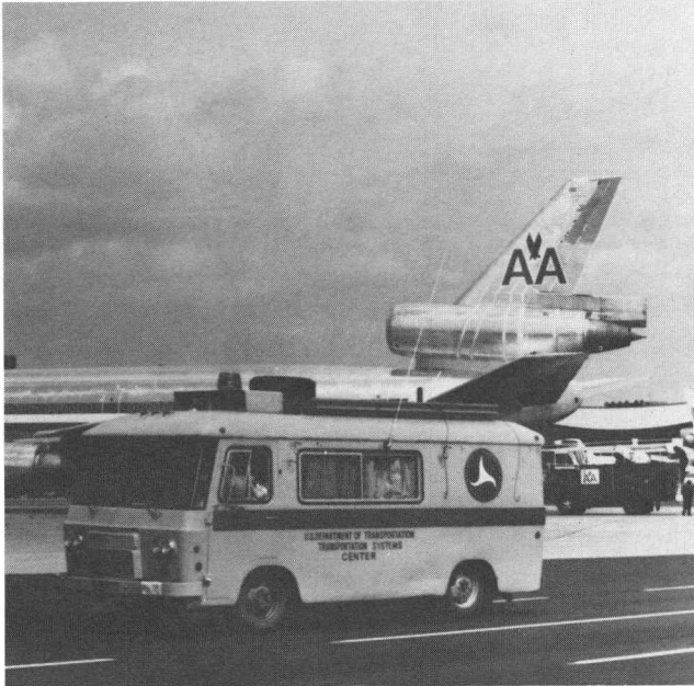
Fig. 1 Traversing the highways with their mobile data acquisition van, which includes a 4051 Graphic System, the U.S. Department of Transportation is evaluating the use of LORAN-C signals for on-land site location.
