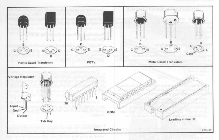
Fig. 5-4. Pin configuration for semiconductor components.
