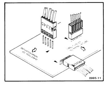
Fig. 5-1. Multipin (harmonica) connector configuration.
