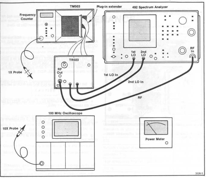
Fig. 4-2. Setup for Adjustment Procedure.
