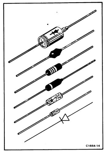
Fig. 5-3. Diode polarity markings.
