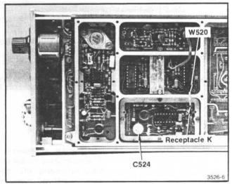
Fig. 4-3. Location of Receptacle K, W520, and C524.
