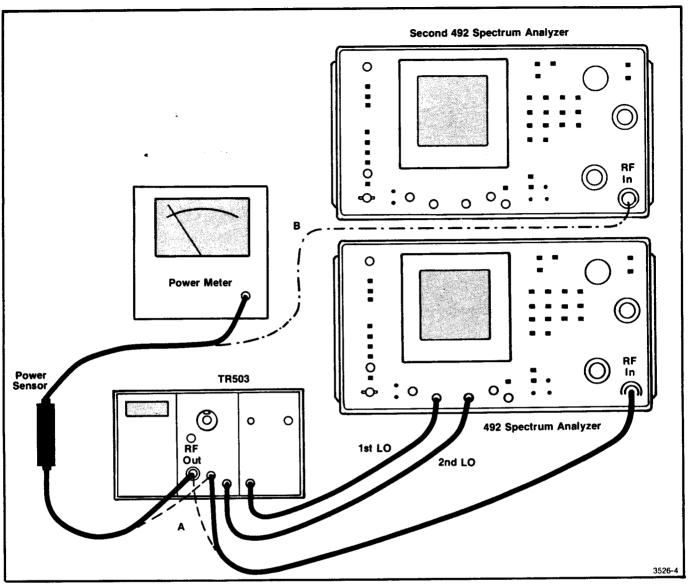
Fig. 4-1. Setup for Performance Check.
