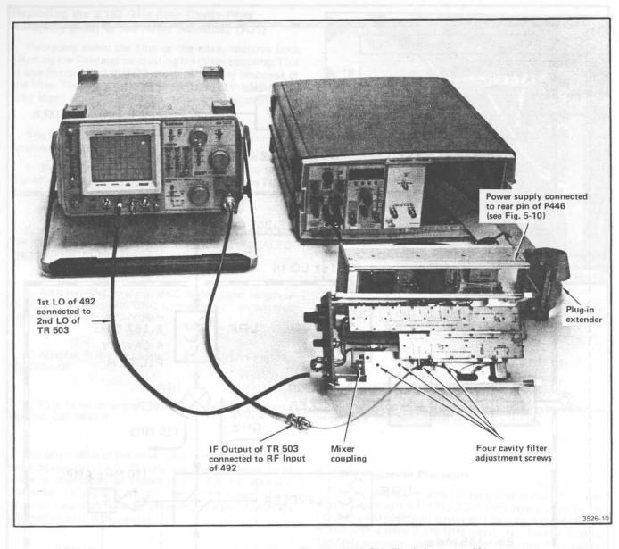
Fig. 5-8. Positioning the TR 503 to adjust the 2.182 GHz filter/mixer assembly.
