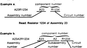
Read: Resistor 1234 of Subassembly 2 of Assembly 23
