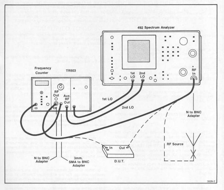
Fig. 2-2. TR 503/492 System with Frequency Counter.
