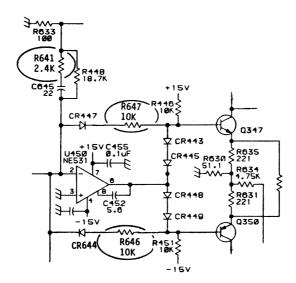
Installation of this modification causes the mainboard part number to change from CM670-6394-00 to CM670-6394-01.
