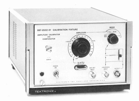
The Amplitude Calibrator and Comparator provides an accurate source for positive and negative DC voltage and current as well as  $60~\mathrm{Hz}$  and  $1~\mathrm{kHz}$  squarewaves. Amplitudes are available from  $0.2~\mathrm{mV}$  to  $100~\mathrm{V}$  in a 1,~2,~5 sequence.
