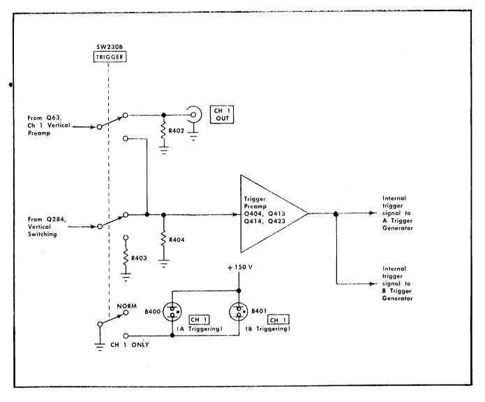
Fig. 3-7. Trigger Preamp detailed diagram
