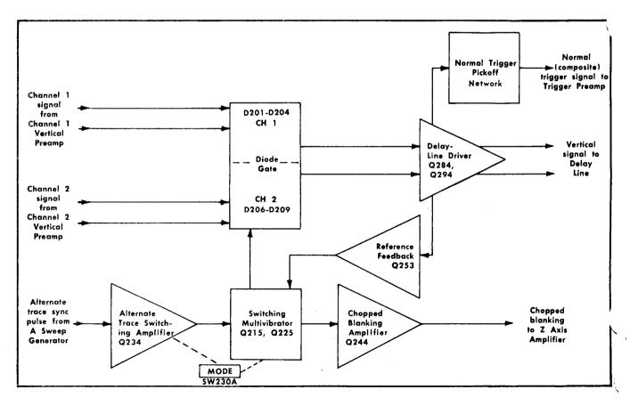
Fig. 3-4. Vertical Switching detailed block diagram.
