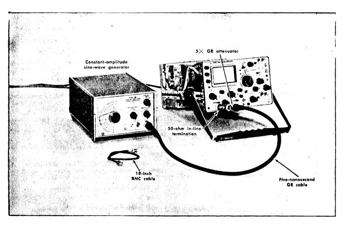
Fig. 6-23. Initial test equipment setup for steps 25 through 27.
