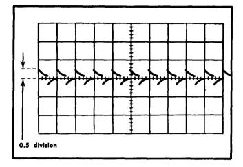
Fig. 5-32. Typical CRT display when checking calibrator current.
