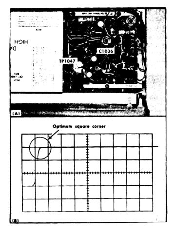
Fig. 6-61. (A) Location of TP1 047 and C1 036, (B) typical tes oscilloscope display showing correct adjustment of C1 036 (vertical deflection, 5 volts/division, sweep rate, 0.1 microsecond/division)
