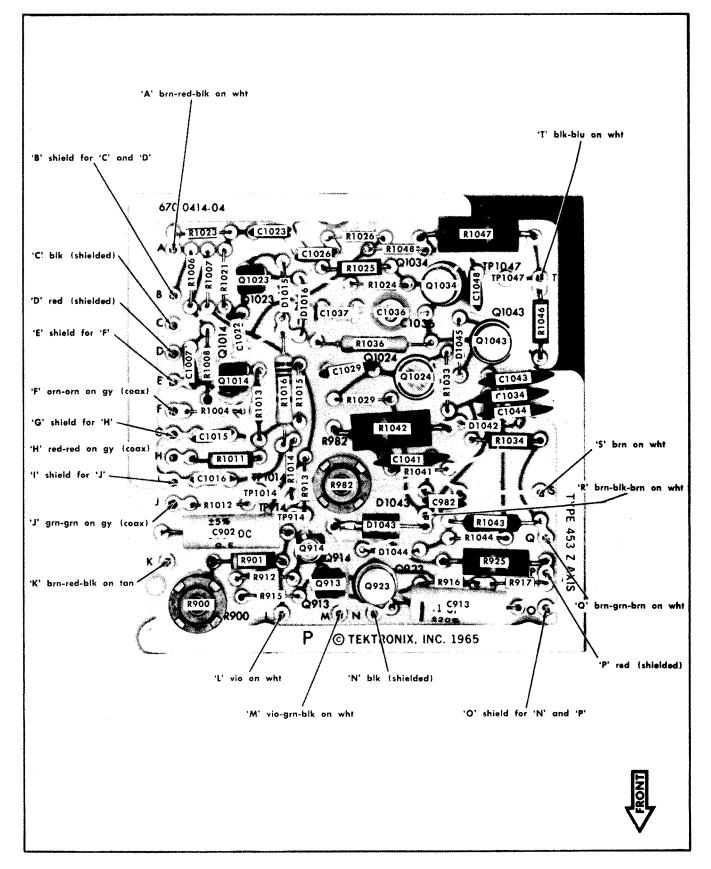
Fig. 4-15. Z Axis Amplifier and High-Voltage Regulator circuit board.
