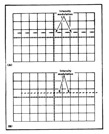
Fig. 6.62. (A) Typical CRT display when checking Z-axis operation at 50 kilohertz, (B) typical CRT display when checking Z-axis operation at 50 megahertz.
