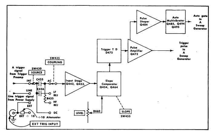
Fig. 3-8. A Trigger Generator detailed block diagram.
