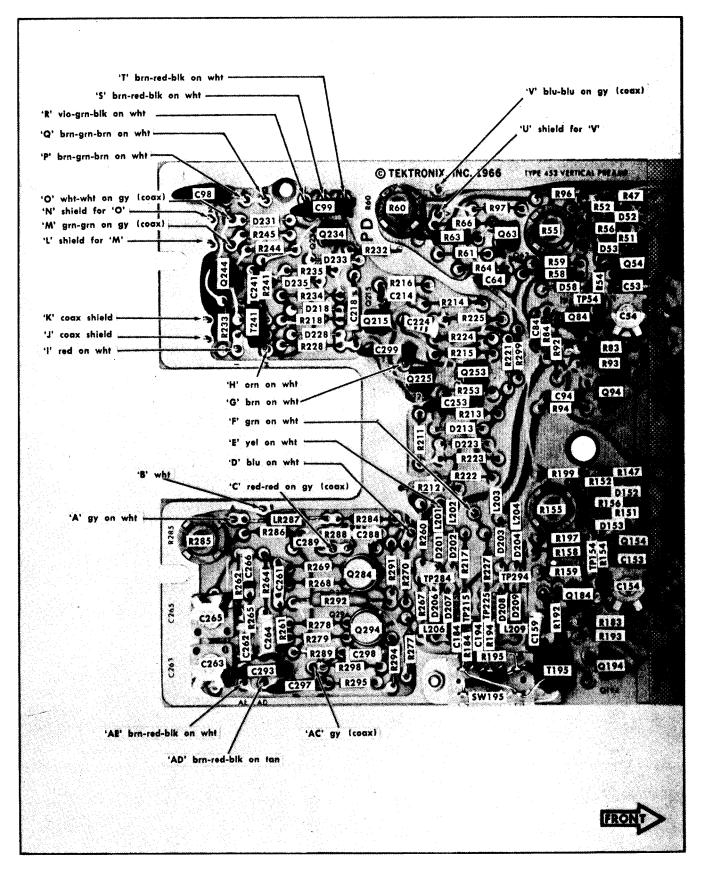
Fig. 4-9. Partial Vertical Preamp circuit board. Vertical Switching and partial Vertical Preamp circuit shown.
