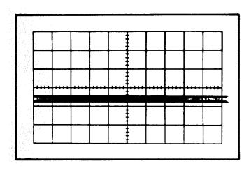
Fig. 5-8. Typical CRT display showing correct common-mode rejection ratio.
