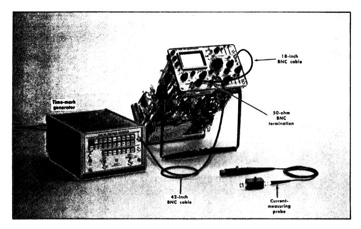
Fig. 6-55. Initial test equipment setup for steps 67 through 70.
