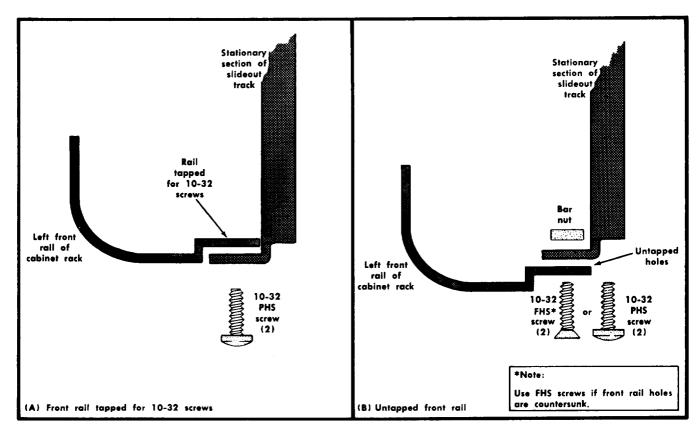
Fig. 10-5. Methods of mounting the stationary section to the front rails.
