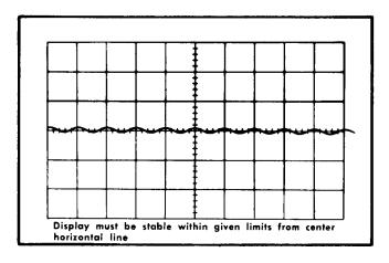
Fig. 5-10. Typical CRT display when checking trigger level centering.
