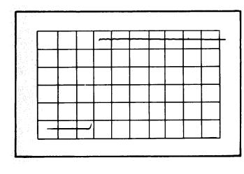
Fig. 5-6. Typical CRT display showing correct high-frequency cominsation. k. Set the MODE switch to CH 2.
