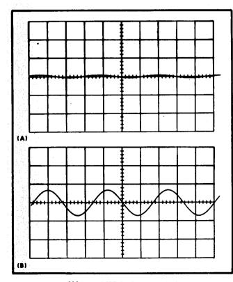
Fig. 6-33. (A) Typical CRT display when checking internal lowrequency triggering at 60 hertz, (B) typical CRT display when hecking external low-frequency triggering 'at 60 hertz.
