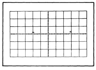
Fig. 5-24. Typical CRT display showing correct X Gain.
