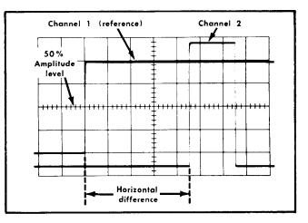
Fig. 2-19. Measuring time difference between two pulses.
