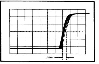
Fig. 2-23. Measuring pulse jitter.
