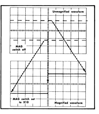
Fig. 2-11. Operation of sweep magnifier.
