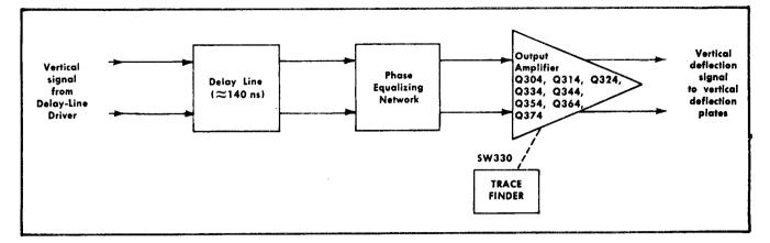
Fig. 3-6. Vertical Output Amplifier detailed block diagram
