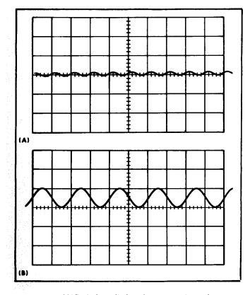
Fig. 5-11. (A) Typical CRT display when checking internal 10-megaintz triggering, (B) typical CRT display when checking internal )-megahertz triggering.
