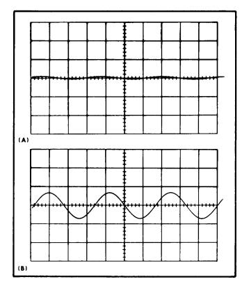
Fig. 5-13. (A) Typical CRT displaay when checking internal low-frequency triggering at 60 hertz. (B) Typical CRT display when checking external low-frequency triggering at 60 hertz.
