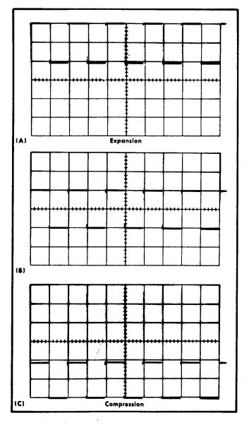
Fig. 6-19. Typical CRT display showing acceptable compression and expansion. (A) Expansion, (B) correct deflection at center of graticule, (C) compression. c. Adjust the Channel 1 VARIABLE control for exactly two divisions of deflection.
