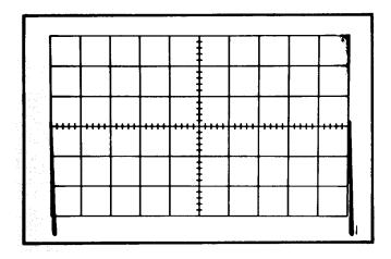
FIg. 5-18. Typical CRT display when checking delayed-sweep actracy.
