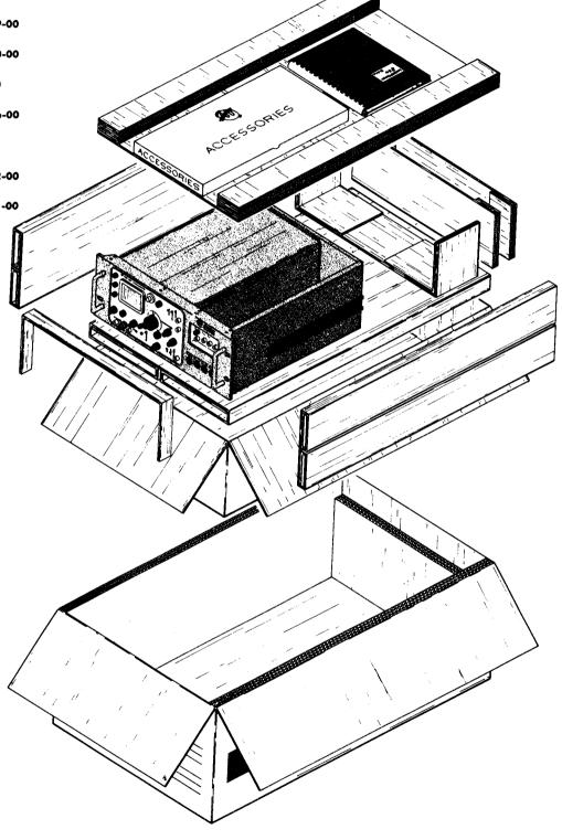
Fig. 4-6. Repackaging the Type R453 for shipment.
