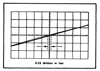
Fig. 6-52. Typical CRT display when checking X-Y phasing.
