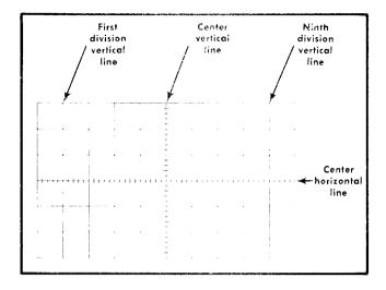
Fig. 2-6. Definition of measurement lines on Type 453 graticule.
