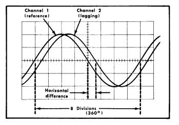
Fig. 2-24. Measuring phase difference.
