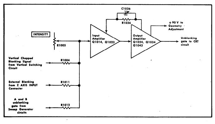
Fig. 3-15. Z Axis Amplifier detailed block diagram.
