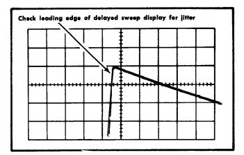
Fig. 6-49. Typical CRT display when checking delay-time jitter.
