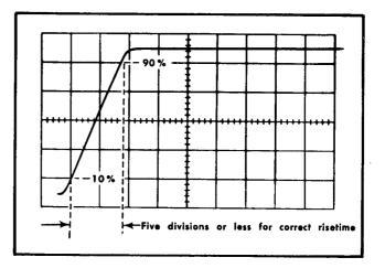
Fig. 5-30. Typical CRT display when checking calibrator risetime.
