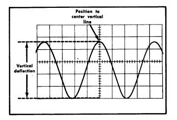
Fig. 2-15. Measuring peak-to-peak voltage of a waveform.
