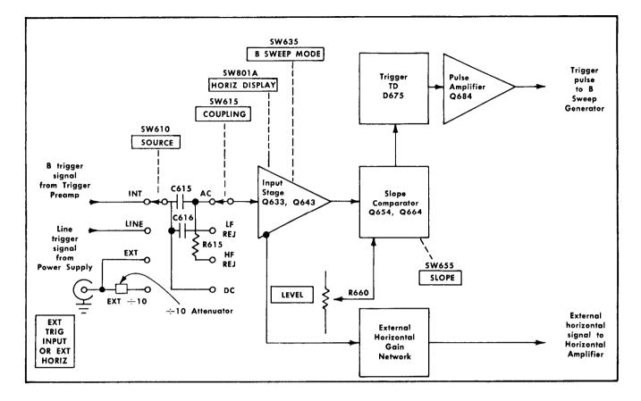
Fig. 3-12. B Trigger Generator detailed block diagram.
