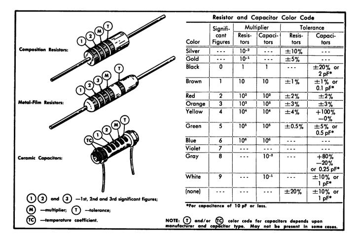
Fig. 4-1. Color code for resistors and ceramic capacitors.
