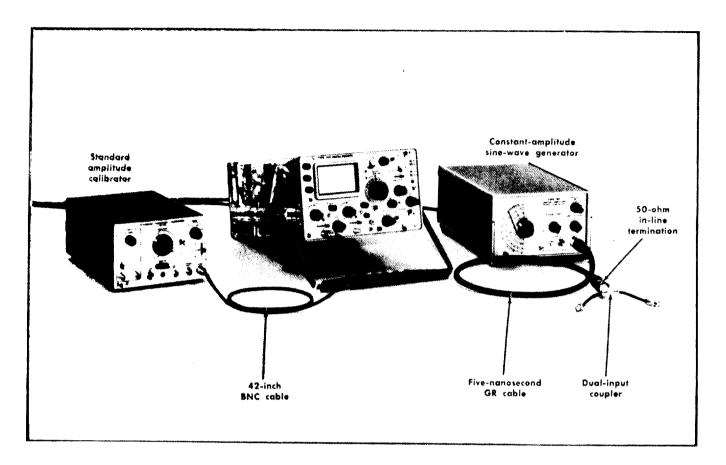
Fig. 6-50. Initial test e quipment setup for steps 61 through 66.
