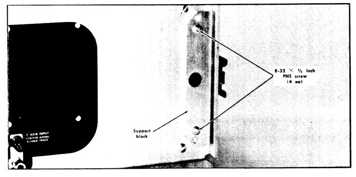
Fig. 10-8. Installing the support black on the Instrument.
