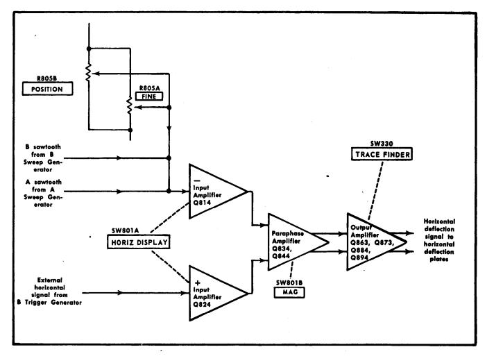
Fig. 3-14. Horizontal Amplifier detailed block diagram.
