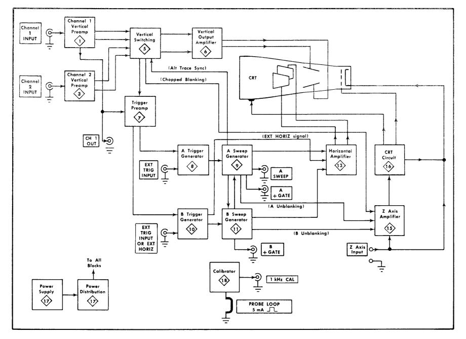
Fig. 3-1. Basic block diagram of the Type 453.
