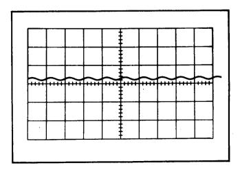
Fig. 6-34. Typical CRT display when checking high-frequency reject operation at 50 kilohertz.
