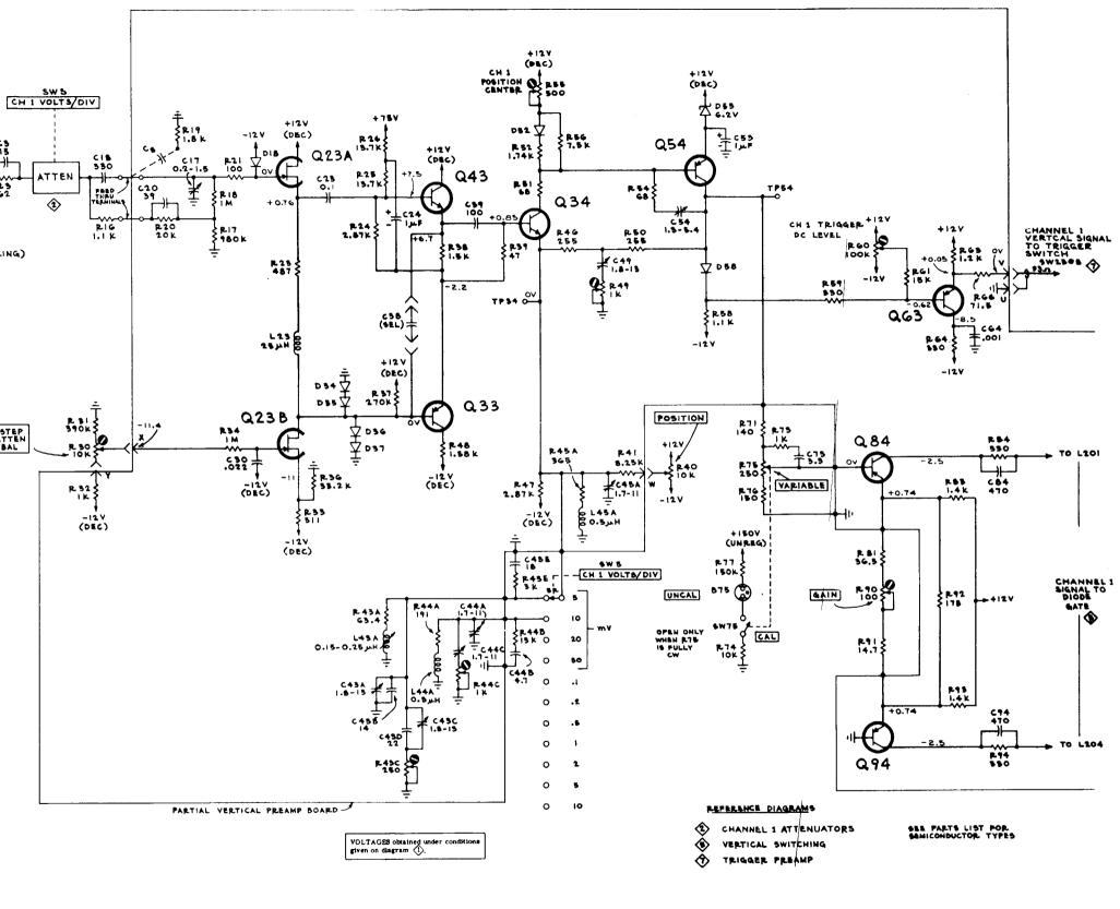
FIG. FO-11. CHANNEL 1 VERTICAL PREAMP
