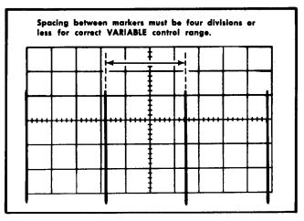
Fig. 5-23. Typical CRT display when checking A and B VARIABLE control range.
