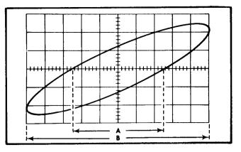
Fig. 2-26. Phase-difference measurement from an X-Y display.
