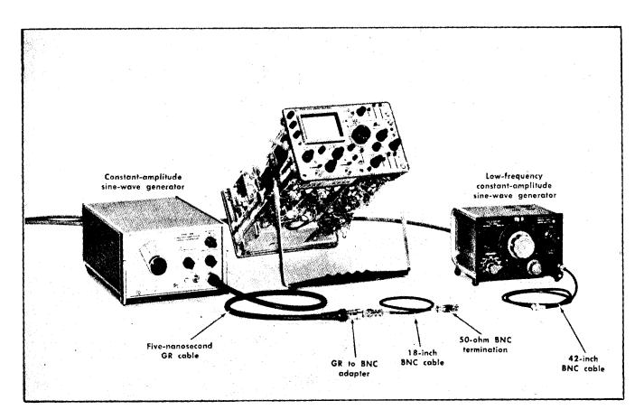
Fig. 6-28. Initial test equipment setup for steps 30 through 40.
