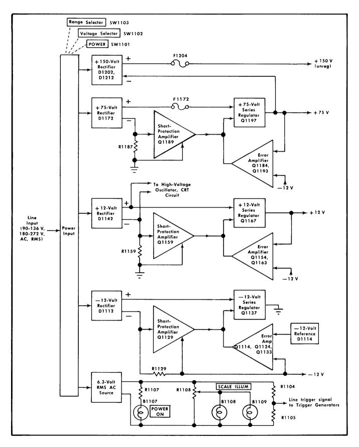
Fig. 3-17. Power Supply detailed block diagram.
