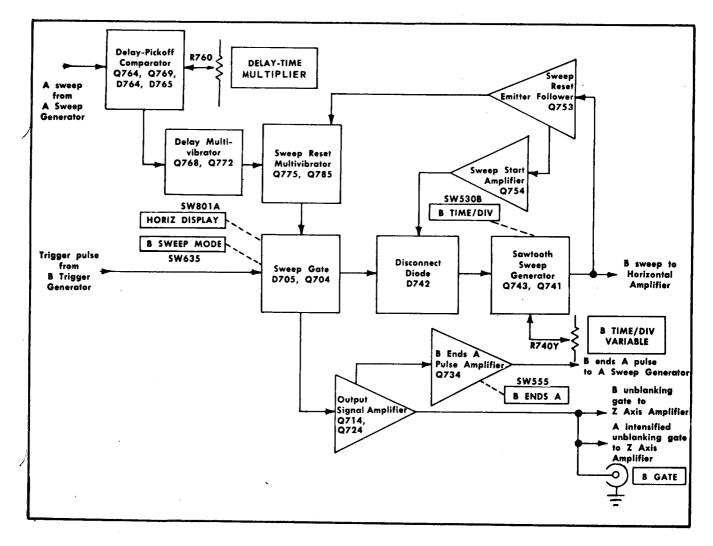
Fig. 3-13. B Sweep Generator detailed block diagram.
