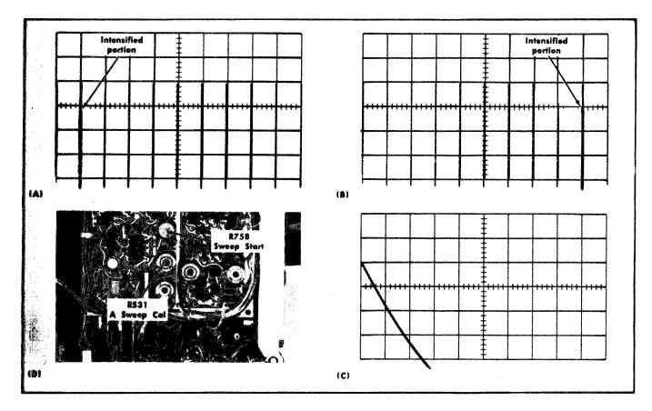
Fig. 6-38. (A) Typical CRT display showing intensified portion correctly located at the second marker, (B) typical CRT display showing intensified portion correctly located at the tenth marker, (C) location of Sweep Start and A Sweep Cal adjustments (B Sweep board), (D) typical CRT display showing correct final adjustment of Sweep Start and A Sweep Cal dajustments.
