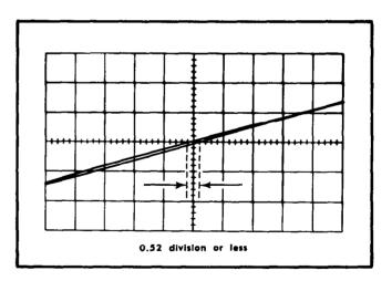
Fig. 5-25. Typical CRT display when checking X-Y phasing.
