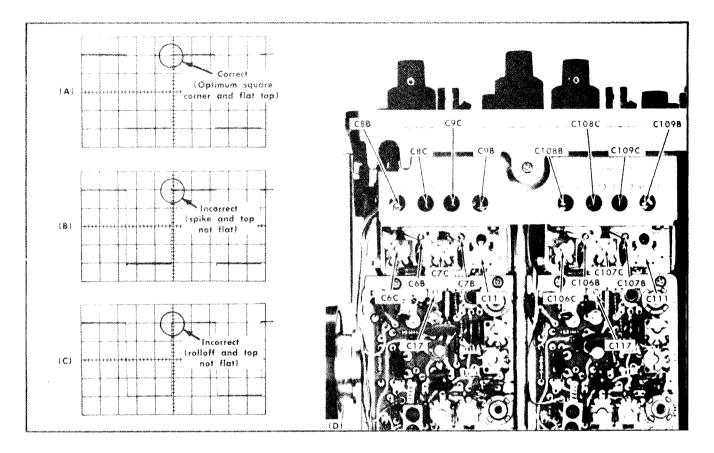
Fig. 6-21. (A) Typical CRT display showing correct compensation; (B) and (C) incorrect compensation; (D) location of variable capacitors (bottom view).
