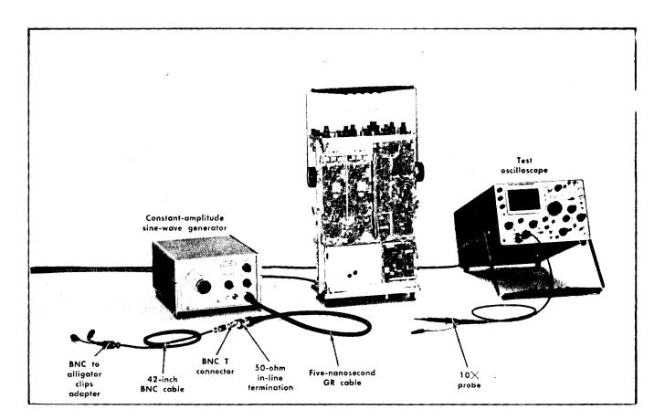
Fig. 6-60. Initial test equipment setup for steps 71 through 74.
