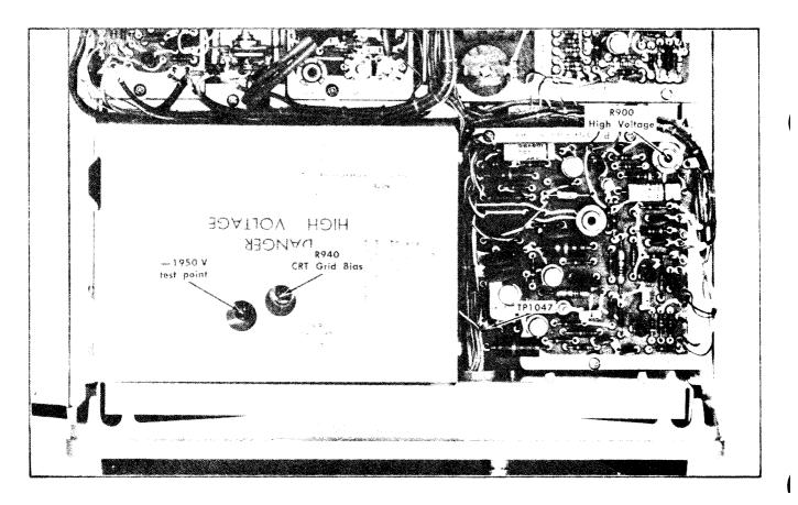
Fig. 6-6. Location of high-voltage adjustments and test points (bottom).
