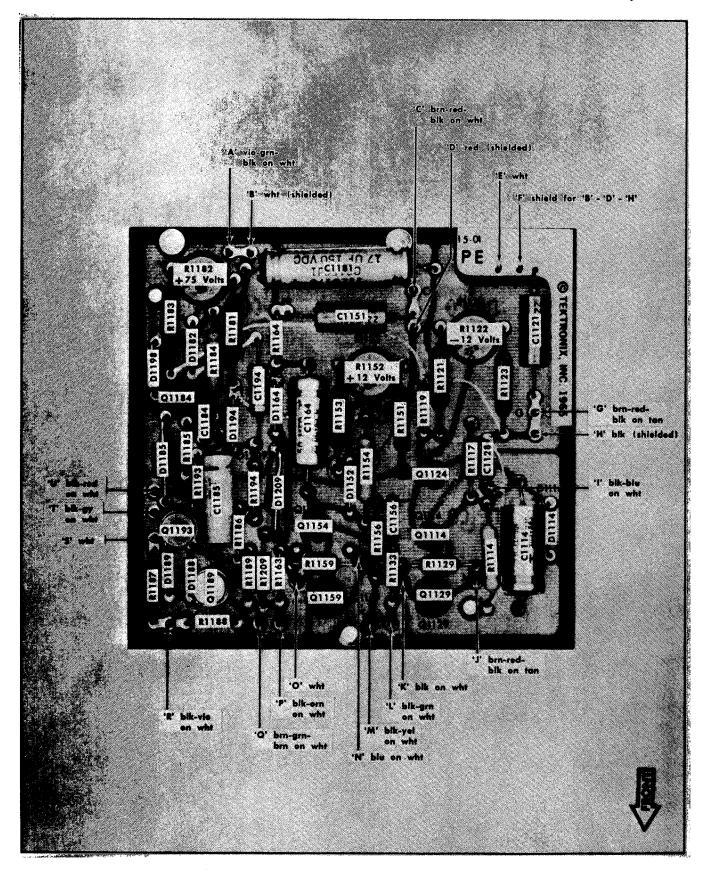
Fig. 4-16. Low Voltage Regulator circuit board.
