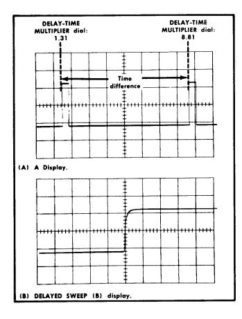
Fig. 2-20. Measuring time difference using delayed sweep.
