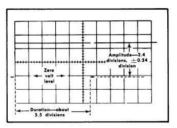
Fig. 5-34. Typical test oscilloscope display when checking A and B GATE output amplitude and duration (vertical deflection factor, five volts/division; sweep rate, two millseconds/division).
