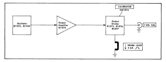
Fig. 3-18. Calibrator detailed block diagram.
