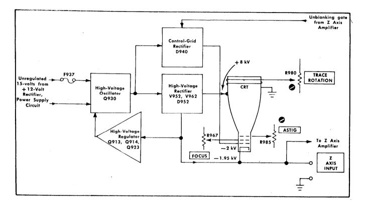
Fig. 3-16. CRT Circuit detailed block diagram.
