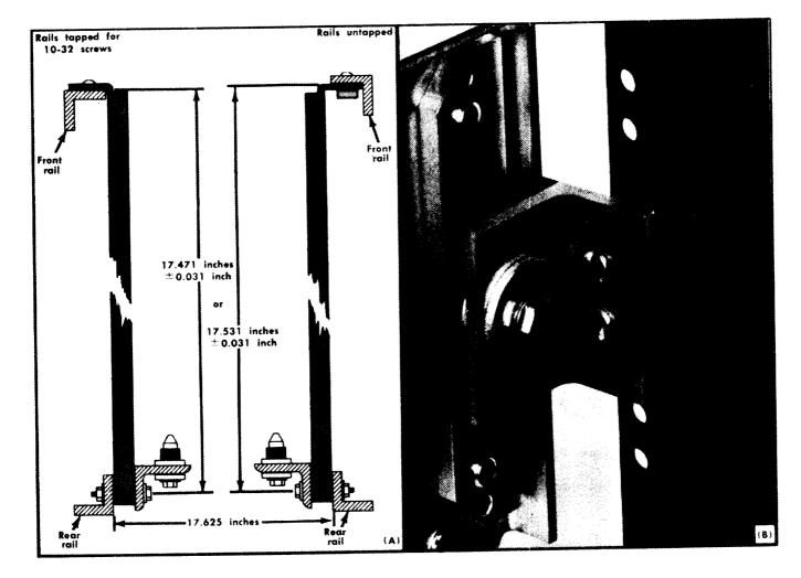
Fig. 10-4. Supporting the rear of the stationary sections: (A) Dimensions necessary; (B) completed installation.
