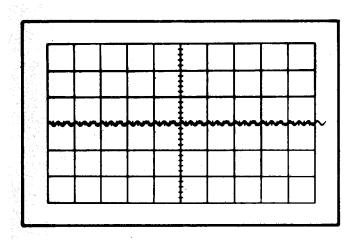
Fig. 5-15. Typical CRT display when checking low-frequency reject eperation at 30 kilohertz.
