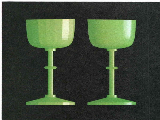
Figure 4. In constant and cosine shading (left), banding is visible. The Gouraud shading (right) generates smooth transitions of colors across an object's surface.
