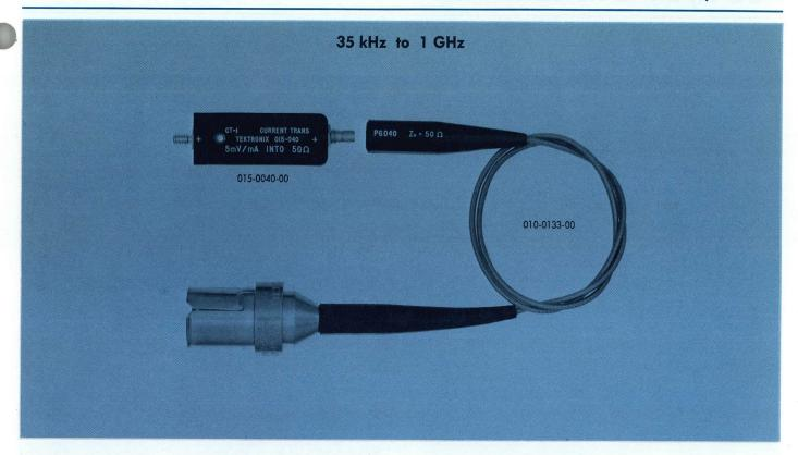
The P6040/CT-1 Current Probe is designed for use with Tektronix 50- $\Omega$  sampling units such as the Tektronix 1S1, 1S2, 3S1, 3S2, 3S5, 3S6 and 7S11 Sampling Plug-In Units. With the use of a 50- $\Omega$  termination the P6040/CT-1 can be used with wideband, non-sampling oscilloscopes for making fast-risetime current measurements.
