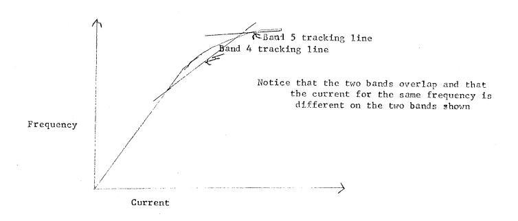
Figure 3 Typical preselector frequency vs. current curve. The nonlinearity of the curve is exaggerated. Typical lines showing current provided by the driver as function of frequency are also shown for bands 4 and 5.
